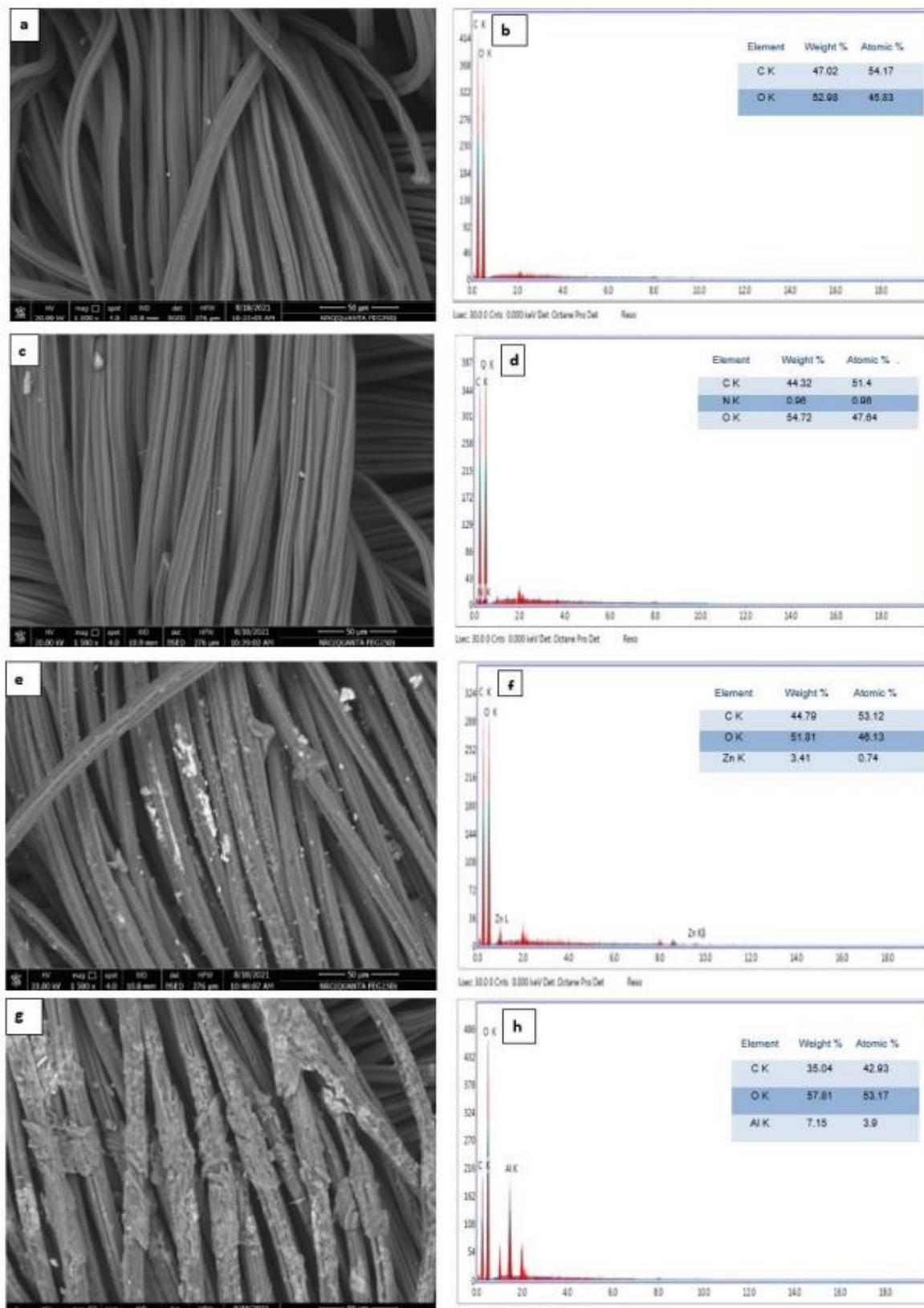
Fig.2. SEM and EDX spectra of untreated viscose samples ( a , b), treated viscose samples with chitosan / CMC (5 / 5 g/L) (c , d), Nano Zinc oxide / CMC (20 / 5 g/L) (e , f) and Nano Aluminum oxide / CMC (20 / 5 g/L) (g , h).
