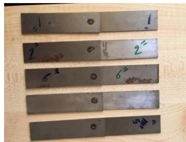
Figure 2. Appearance for resistance spot welding joint.
