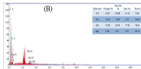
**Figure 12:** EDX spectra of (A) CPVP and (B) CPVP/Ag-NPs hydrogels.
