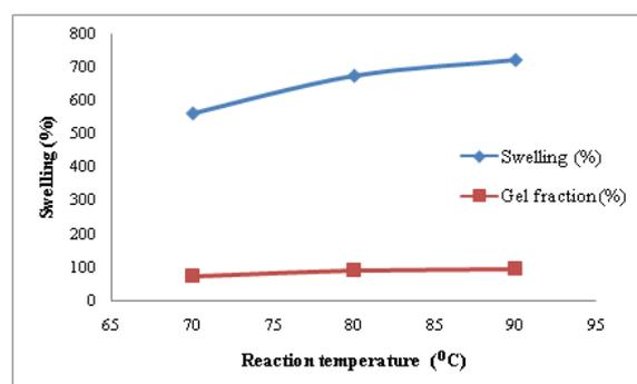
**Figure 4:** Effect of reaction temperature on percent swelling and gel fraction of PVP gel. PVP MW, 40,000; APS/PVP weight ratio, 100%, PVP conc., 65%; reaction time, 60 min. Swelling properties was assessed at pH 7 and 25 °C.
