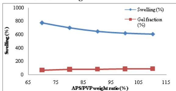
**Figure 2:** Effect of APS/PVP weight ratio on percent swelling and gel fraction of PVP gel. PVP MW, 40,000; PVP conc., 60%; reaction temp., 80 °C; reaction time, 60 min. Swelling properties was assessed at pH 7 and 25 °C.
