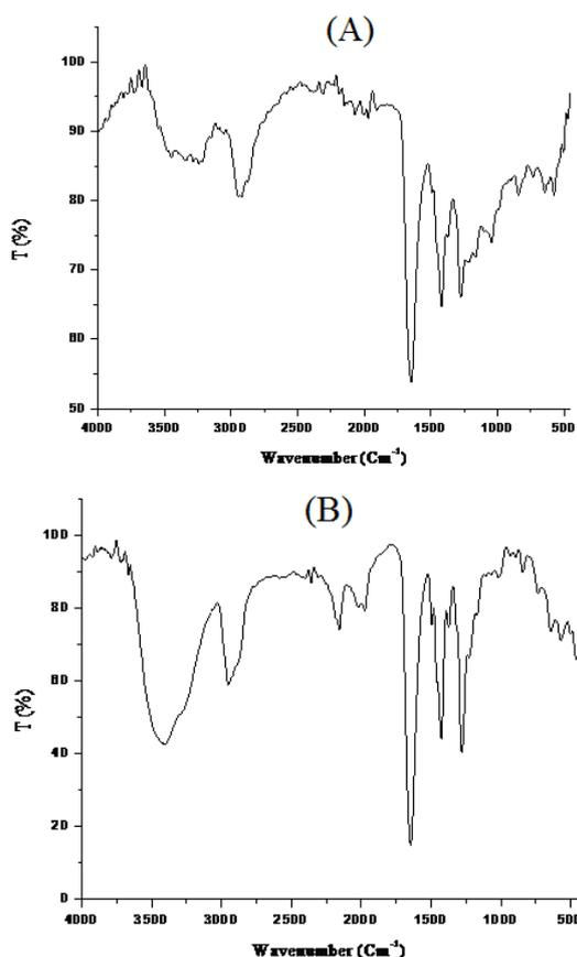
**Figure 8:** FTIR spectra of (A) CPVP and (B) PVP.
