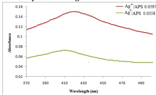
**Figure 9:** UV-Vis absorption spectrum of the synthesized Ag-NPs.
