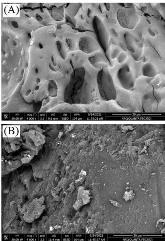
**Figure 11:** SEM images of (A) CPVP and (B) CPVP/Ag-NPs hydrogels.
