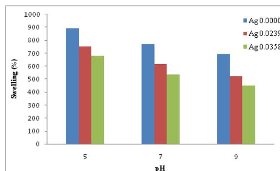
**Figure 7:** Effect of Ag<sup>+</sup>/APS molar ratio on percent swelling of CPVP/Ag-NPs nanocomposite at different pHs. PVP MW, 40,000 Da; APS/PVP weight ratio, 100%, PVP conc., 65%; reaction temp., 90°C; reaction time, 40 min; pH, 2.5. Swelling properties was assessed at 25 °C.
