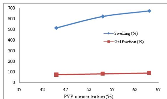
**Figure 3:** Effect of PVP concentration on percent swelling and gel fraction of PVP gel. PVP MW, 40,000; APS/PVP weight ratio, 100%, reaction temp., 80 °C; reaction time, 60 min. Swelling properties was assessed at pH 7 and 25 °C.
