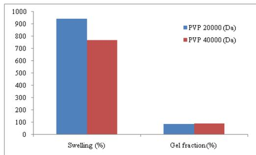
**Figure 6:** Effect of PVP molecular weight on percent swelling and gel fraction of PVP gel. APS/PVP weight ratio, 100%, PVP conc., 65%; reaction temp., 90°C; reaction time, 40 min. Swelling properties was assessed at pH 7 and 25 °C.
