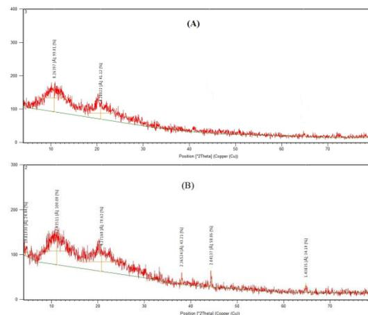
**Figure 10:** XRD pattern of (A) CPVP and (B) CPVP/Ag-NPs.
