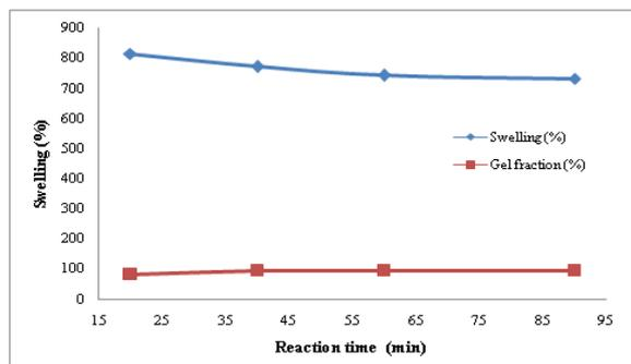
**Figure 5:** Effect of reaction time on percent swelling and gel fraction of PVP gel. PVP MW, 40,000; APS/PVP weight ratio, 100%, PVP conc., 65%; reaction temp., 90°C. Swelling properties was assessed at pH 7 and 25 °C.
