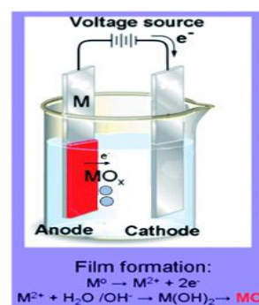
Fig. 1: Schematic illustration showing a simplified anodization cell [6].
