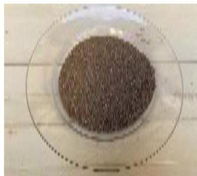
Fig 6. Prepared Sewage sludge (adsorbent).
