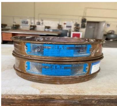
Fig 5. Sieves 1.18mm and 0.6mm
