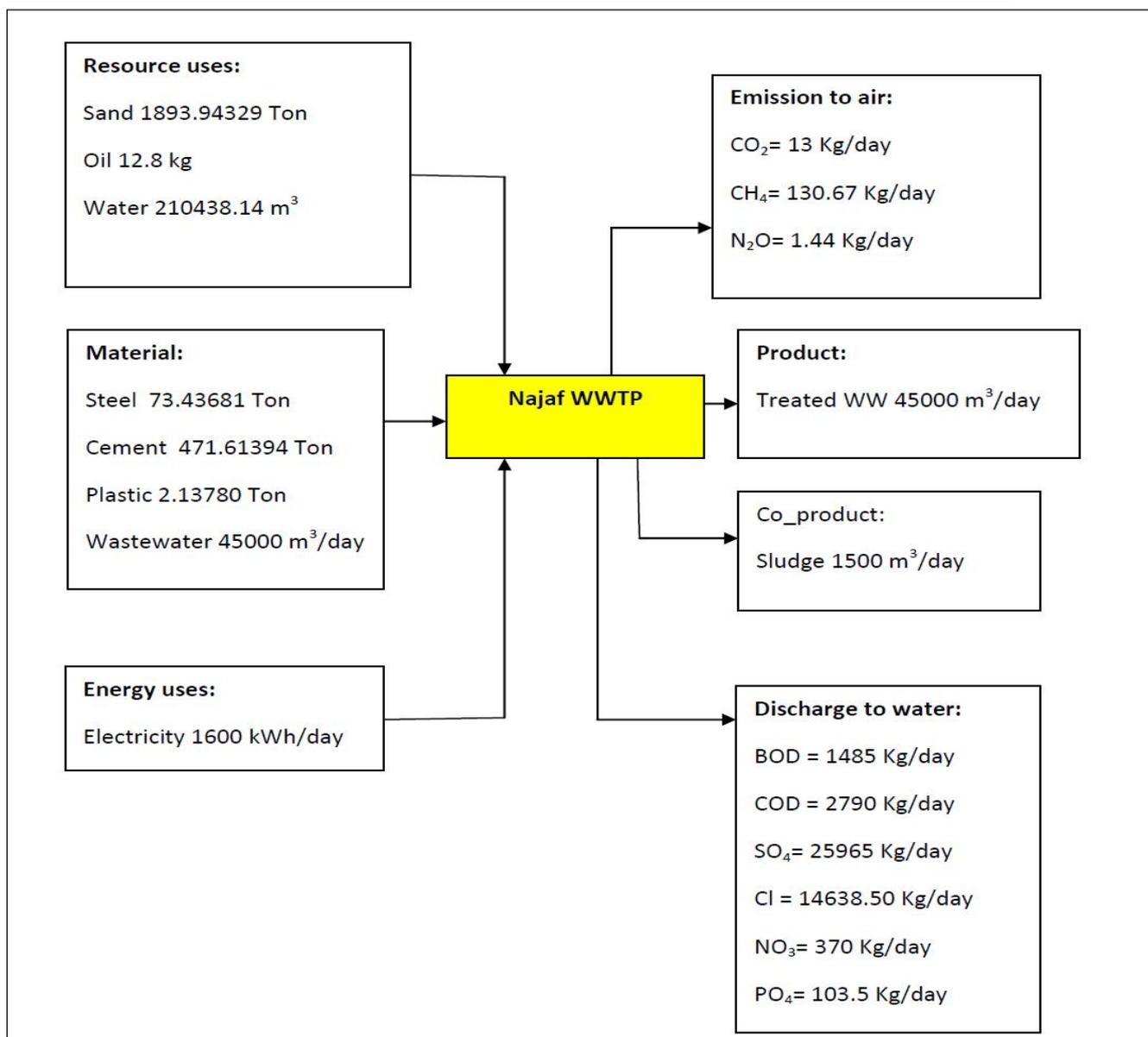
Fig 4 Inventory analysis of Najaf wastewater treatment plant [16].
