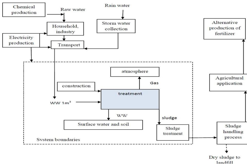
Fig.2: System boundaries for wastewater treatment system ( Modified from) [14].
