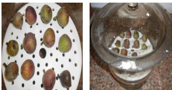
**Figure 2** Fig fruit samples into a sterile glass discator with (90% RH.) before incubation.
