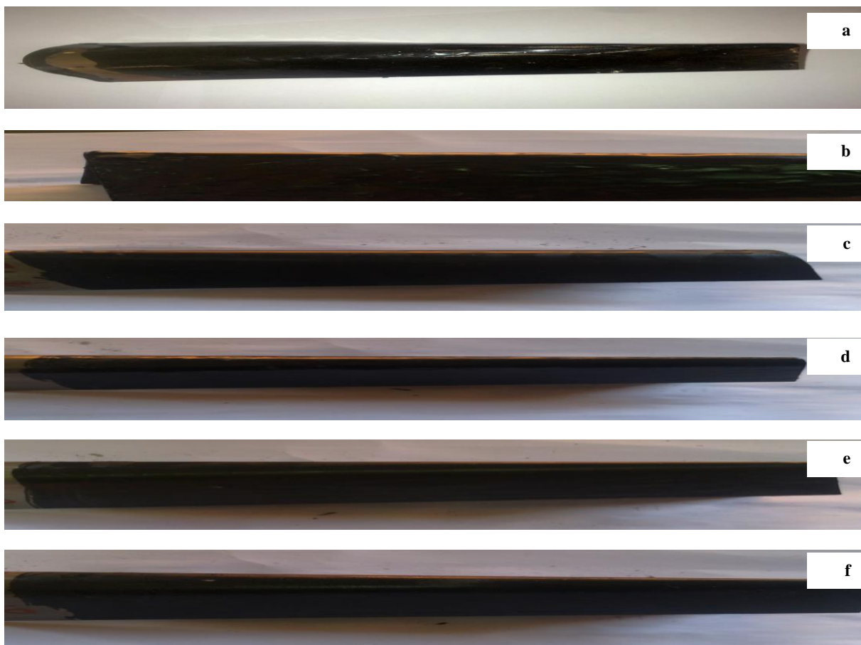
Fig. 9: Mandrel bend testing panel of a) virgin asphalt (Ac), b) Oxidized asphalt, and bioasphalt binder containing c) 2% NCMA, d) 4% NCMA, e) 6% NCMA, and f) 8 % NCMA.
