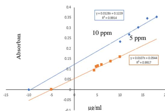
Fig.5 Standard addition method of Metronidazole intravenous injection 500 mg/100ml (Iraq-Sulaymaniyah)
