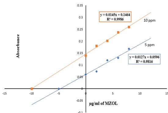
Fig.4 Standard addition method of Metronidazole tablet/250mg (Indian)
