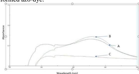
Figure 2. The absorption spectrum of A: MZOL azo dye against blank B: MZOL azo dye against distilled water C: blank against distilled water Recommended procedure and calibration curve
