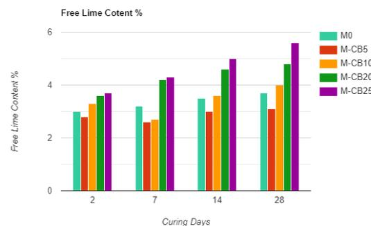
**Figure (7):-** Free lime content of white cement and CB blended cement pastes hydrated for 28 days.
