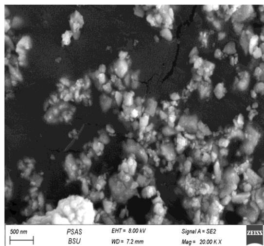
**Figure (2):-** SEM morphology & Microstructure of clay brick powder after milling process.
