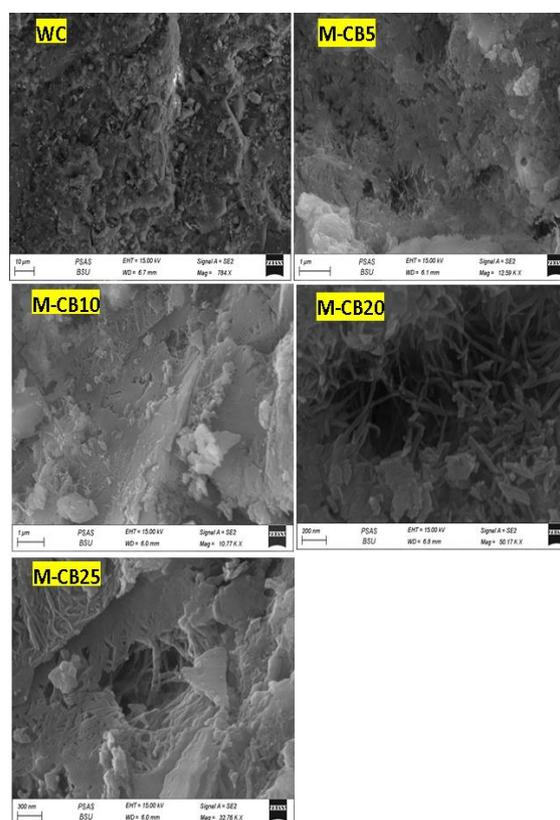
**Figure (9):-** Hydration and microstructure of white cement and CB blended cement pastes hydrated for 28 days
