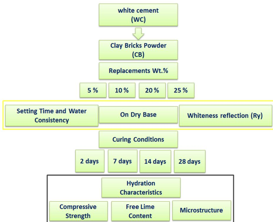
**Figure (3):-** Schematic diagram for experimental program.
