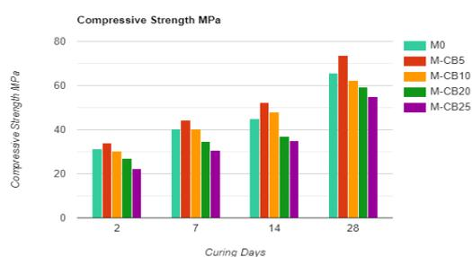
**Figure (8):-** Compressive Strength of white cement and CB blended cement pastes hydrated for 28 days.
