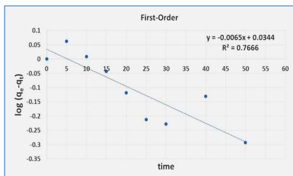
Figure 13. Pseudo-first order adsorption kinetics of Cr (VI) onto MNPs.
