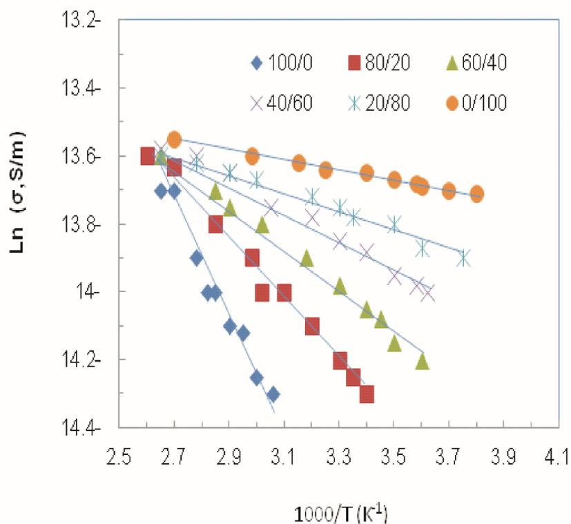
Fig. 8. Dependence of  $\sigma_{ac}$  on temperature of vulcanized SBR/NBR blends at 100 kHz.
