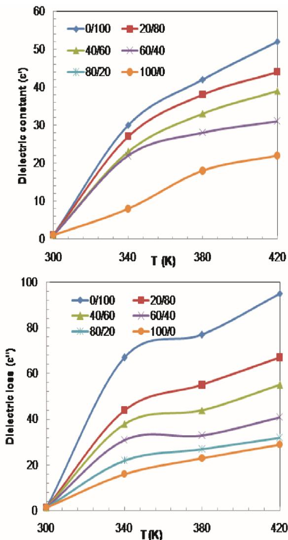
Fig. 12. The temperature dependence of the dielectric properties (dielectric constant/permittivity and dielectric loss) of vulcanized SBR/NBR blends at 100 kHz.
