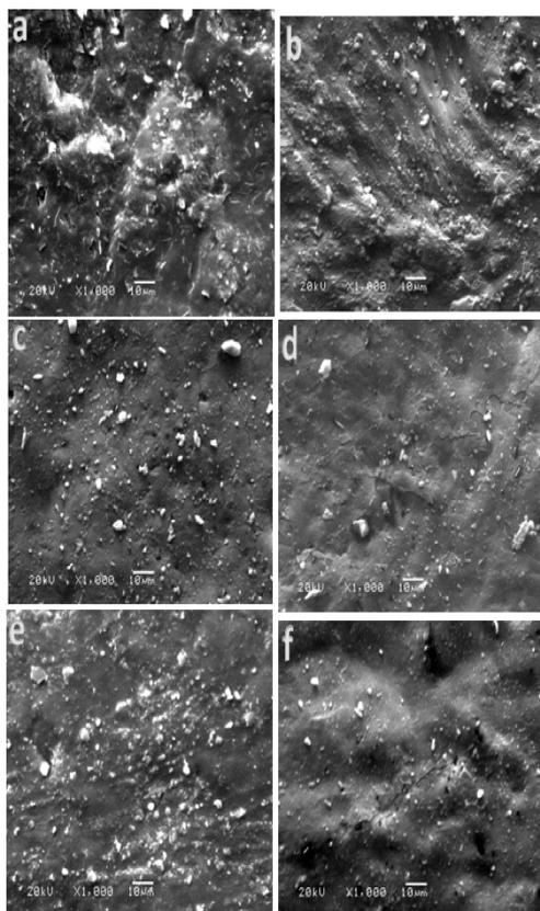
**Fig. 1.** SEM micrographs of vulcanized SBR/NBR blends as (0/100, 20/80, 40/60, 60/40, 80/20 and 100/0) of (a, b, c, d, e, and f), respectively.
