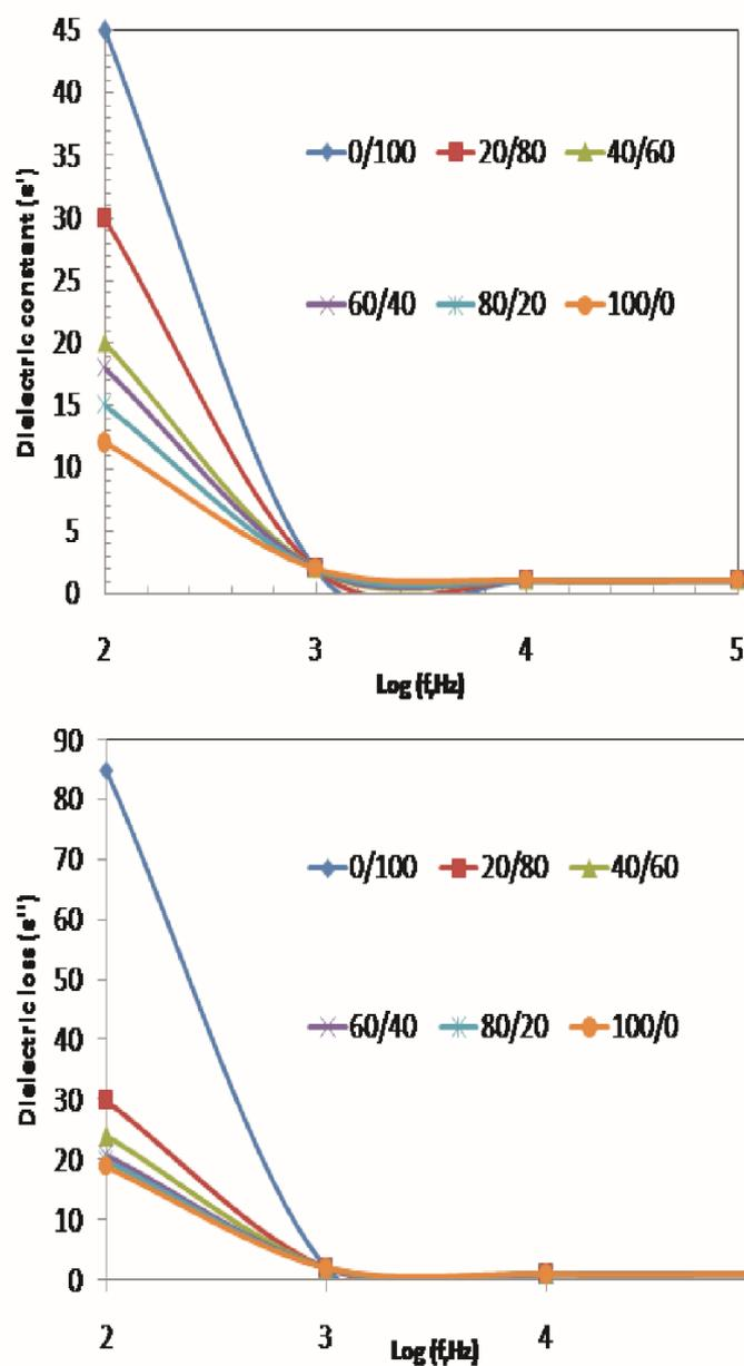
Fig. 11. The frequency dependence of the dielectric properties for dielectric constant/permittivity, and dielectric loss of for vulcanized SBR/NBR blends at 300K.
