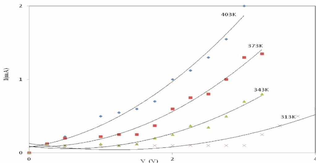
Fig. 9. Current-voltage characteristics at different temperatures for vulcanized 0SBR/100NBR blend sample.
