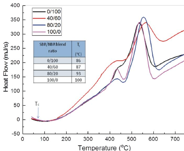
Fig. 3. DSC thermograms of vulcanized SBR/NBR blends as a function of SBR/NBR ratio in blend system.
