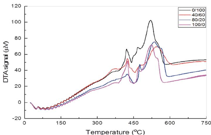
**Fig. 2.** DTA thermograms of vulcanized SBR/NBR blends as a function of SBR/NBR ratio in blend system.
