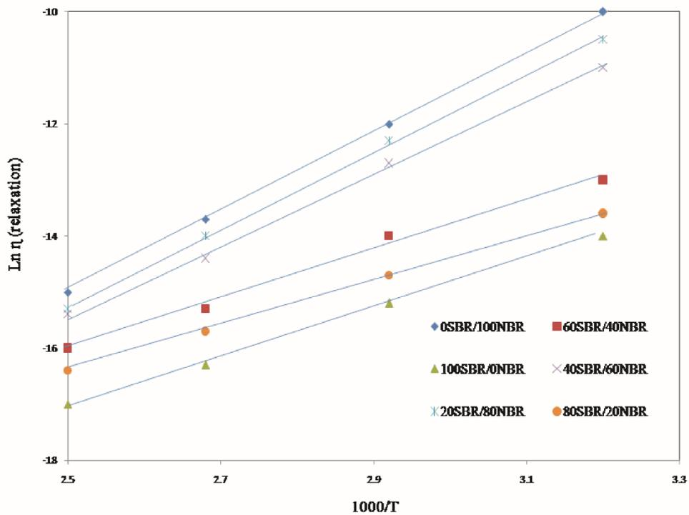
Fig. 5. Relaxation time versus  $1000/T$  of all investigated rubber vulcanized blend sample.
