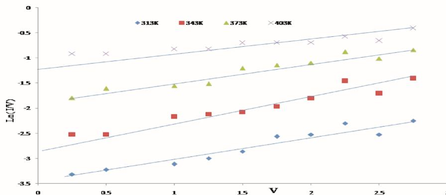
Fig. 10 Ln (I/V) versus V at different temperature for vulcanized 0SBR/100NBR blend sample.
