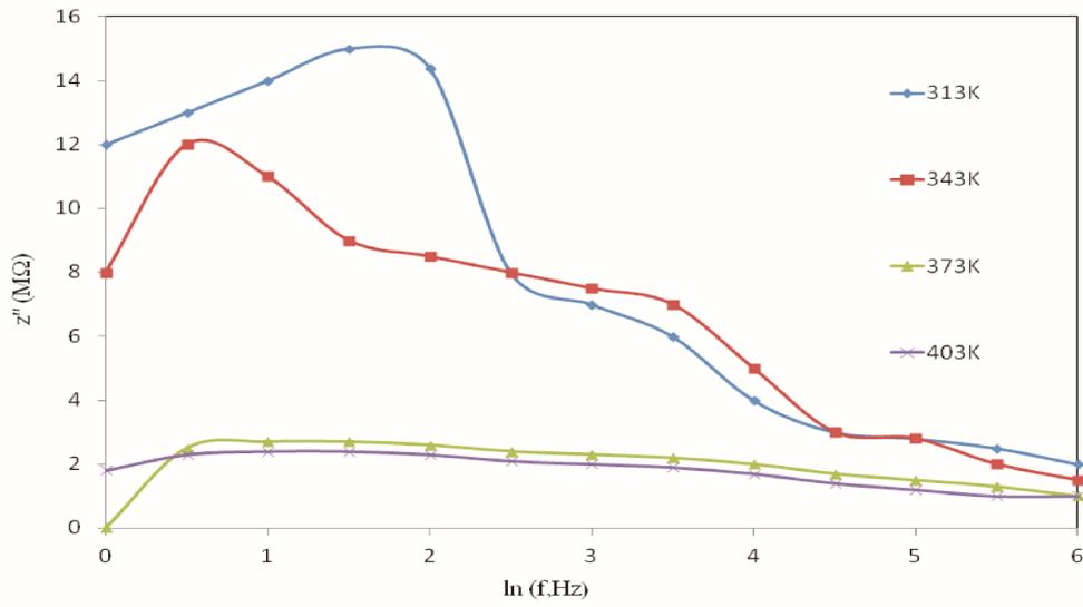
Fig. 4. Dependence of  $Z''$  on frequency for the blends within different temperature ranges.
