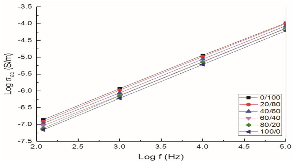
Fig. 6. AC electrical conductivity of SBR/NBR blends versus frequency at room temperature, (300K).
