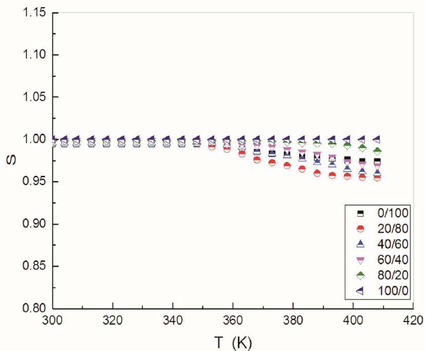
Fig. 7. Dependence of s exponent on temperature of vulcanized SBR/NBR blends.
