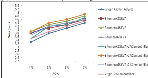
Fig (B): Marshall curves of Flow t
