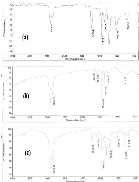
Fig. (4): FTIR spectra of (a) WEVA (b) Virgin asphalt (c) WEVA modified asphalt
