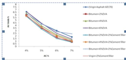
Fig(C): Marshall Curves of Air Voids
