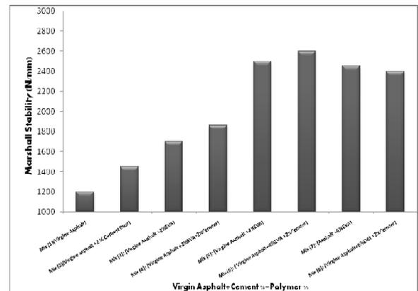
Fig (9) : Effect of polymer type and content on the stability of the prepared mixes.
