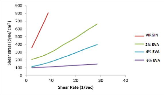
Figure (6): Shear stress- shear rate curves of PMA using EVA at 60°C.
