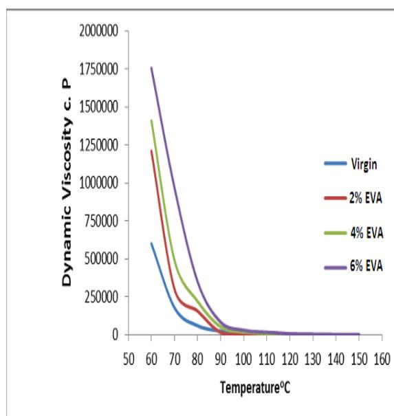
Figure (5): Dynamic viscosity with temperature of PMA using EVA Waste.
