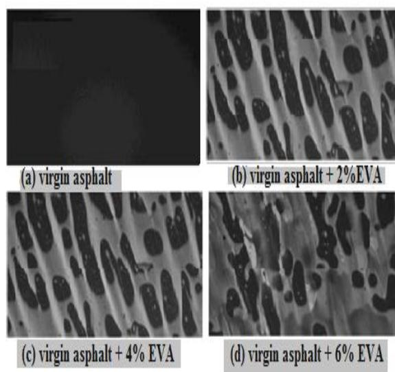
Fig. (3): SEM photo of AC virgin and 2%, 4% and 6% Waste EVA modified asphalt
