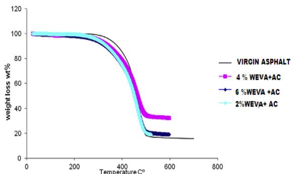
Fig. (2): TGA curves of AC virgin and 2%, 4% and 6% Waste EVA modified asphalt.
