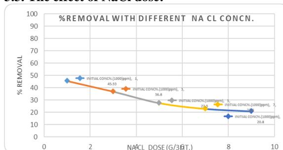
Figure (5): The Effect of NaCl Dose on % Removal ( $C_o=1000$  ppm, rpm =750)
