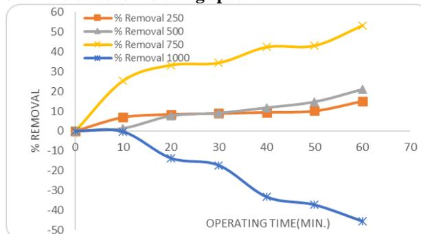
Figure (4): The Effect of Rotating Speed (rpm) on % Removal ( $C_o=1000$  ppm)
