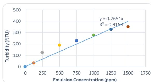
Figure (3): Emulsion Concentration Calibration Curve Using NTU of the Turbidity Meter
