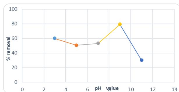
Figure (6): The Effect of pH on % Removal (C<sub>0</sub>=1000 ppm, r.p.m =750)
