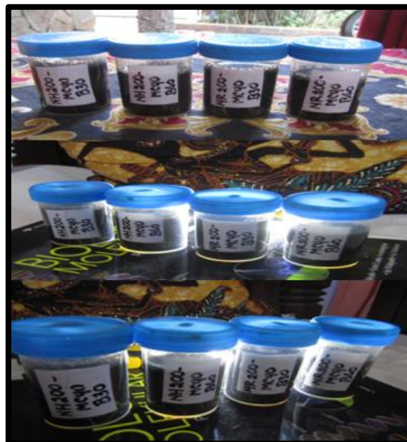
Figure 7. The colloid of CNMs from patchouli biomass by hydrothermal - microwave (NH200-MC40) and reflux - microwave (NR200-MC40) methods after blending process for 30 minutes (B30) and 60 minutes (B60) under sunshine and the flash light.
