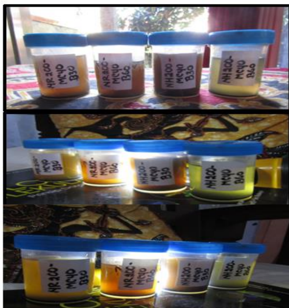
Figure 11. The colloid of CNMs from patchouli biomass by hydrothermal - microwave (NH200-MC40) and reflux - microwave (NR200-MC40) methods after blending process for 30 minutes (B30) and 60 minutes (B60) under the flah light after keeping for 26.75 h.
