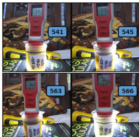
Figure 12. TDS measurement process for the colloid of CNMs from patchouli biomass by hydrothermal - microwave (NH200-MC40) and reflux - microwave (NR200-MC40) methods after blending process for 30 minutes (B30) and 60 minutes (B60) after keeping for 26.75 h.
