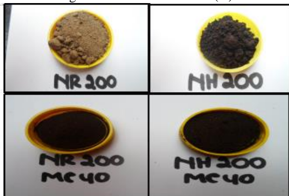
Figure 2. Biomass (N) and the carbon from pyrolysis of patchouli biomass using reflux–microwave (NR200-MC40) and hydrothermal–microwave (NH200-MC40).
