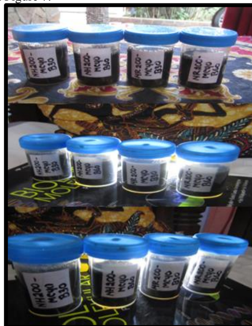
Figure 7. The colloid of CNMs from patchouli biomass by hydrothermal - microwave (NH200-MC40) and reflux - microwave (NR200-MC40) methods after blending process for 30 minutes (B30) and 60 minutes (B60) under sunshine and the flash light.
