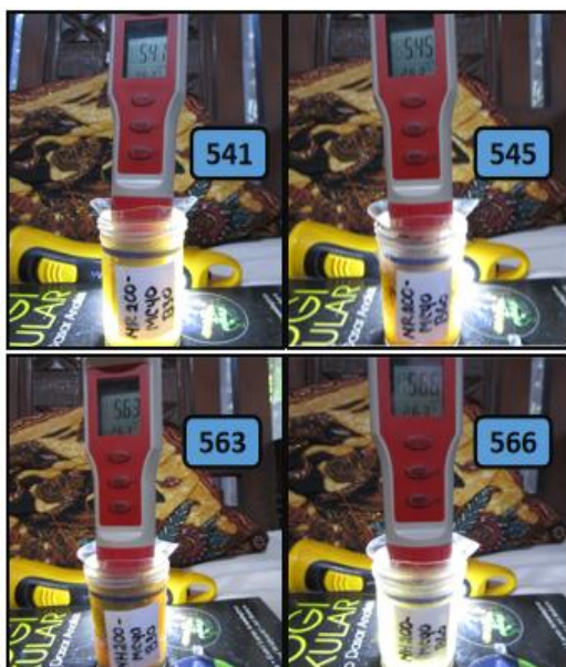
Figure 12. TDS measurement process for the colloid of CNMs from patchouli biomass by hydrothermal - microwave (NH200-MC40) and reflux - microwave (NR200-MC40) methods after blending process for 30 minutes (B30) and 60 minutes (B60) after keeping for 26.75
