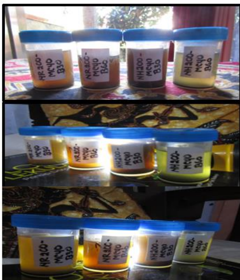
Figure 11. The colloid of CNMs from patchouli biomass by hydrothermal - microwave (NH200-MC40) and reflux - microwave (NR200-MC40) methods after blending process for 30 minutes (B30) and 60 minutes (B60) under the flash light after keeping for 26.75 h.
