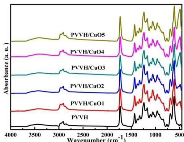
Fig. 3: ATR-FTIR spectra of PVVH incorporated with a different weight percentage of CuO NPs.
