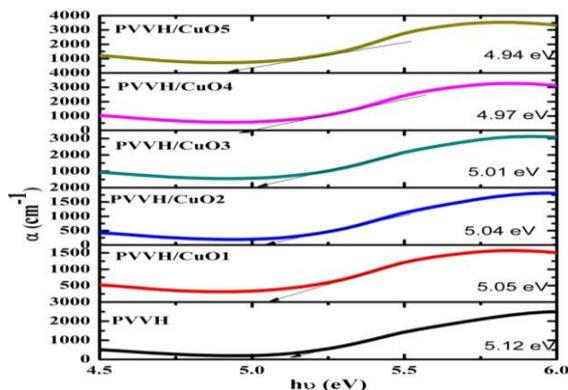
Fig. 5: Relation between absorption coefficient and photon energy of PVVH incorporated with a different weight percentage of CuO NPs.
