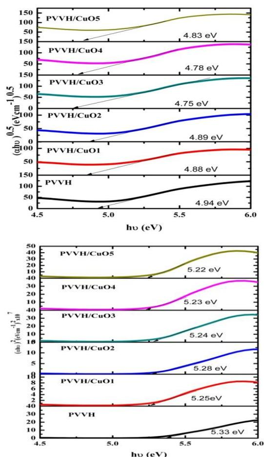
Fig. 7: Relation between  $(\alpha h\nu)^{1/2}$  and  $(\alpha h\nu)^2$  against  $h\nu$  for of PVVH incorporated with a different weight percentage of CuO NPs.
