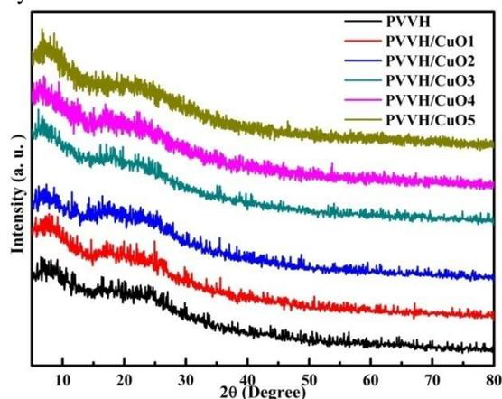
Fig. 1: XRD patterns of PVVH incorporated with different weight percentages of CuO NPs.
