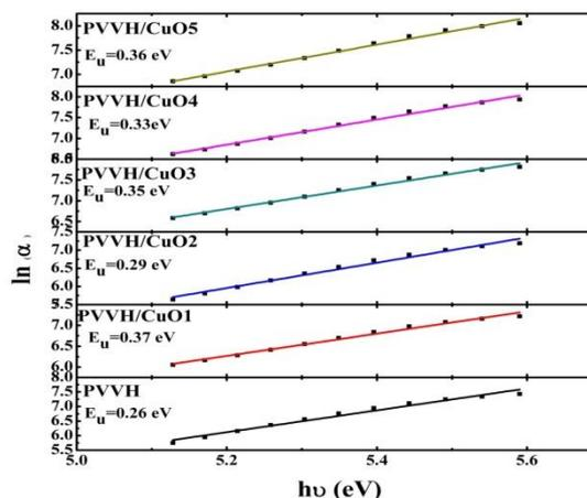
Fig. 6: Relation between  $\ln \alpha$  and  $h\nu$  of PVVH incorporated with a different weight percentage of CuO NPs.
