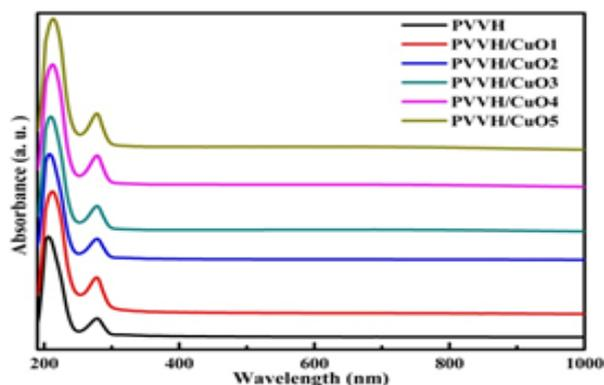
Fig. 4: UV-Vis of PVVH incorporated with a different weight percentage of CuO NPs.
