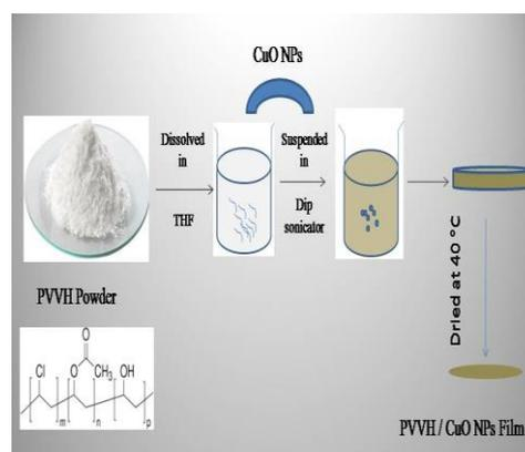
Scheme 1: Steps of preparation of PVVH/ (wt%) CuO NPs.
