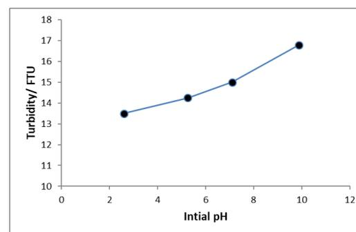
Fig. 8. Relation between initial pH and output Turbidity
