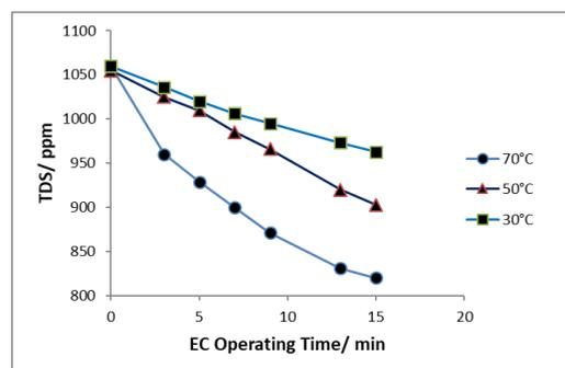
Fig. 7. Relation between time and TDS at different T
