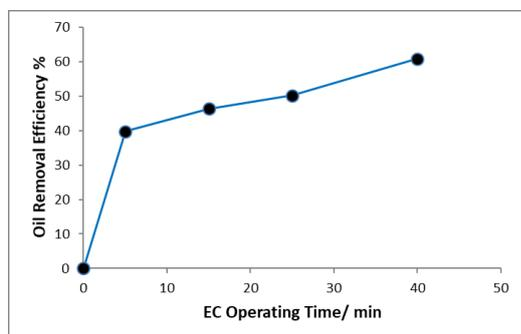
Fig. 5. Relation between time and oil removal
