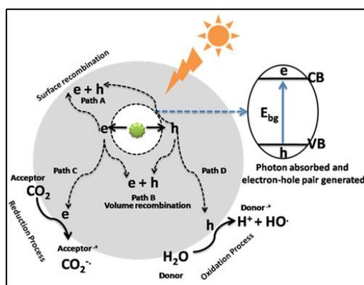
Fig. 1. Schematic diagram of the basic reaction mechanism of a semiconductor photocatalyst.
