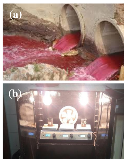
Figure 1 (a) The pink color of the dye effluent wastewater and (b) The photocell used in the dye treatment experiment.
