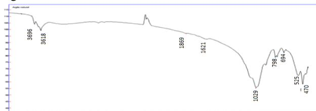
Figure 1: The IR spectrum of clay
