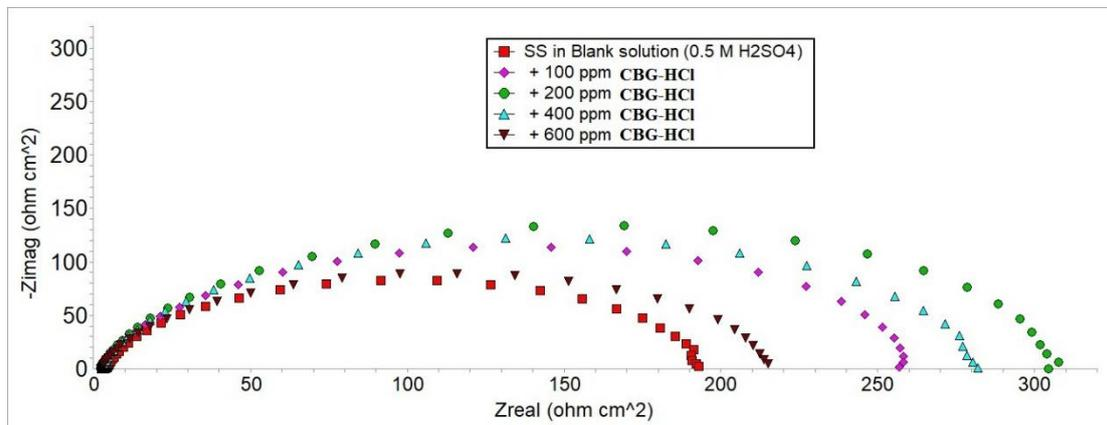
Fig. 2. Nyquist SS plot reported for various CBG-HCl concentrations in 0.5 M  $H_2SO_4$  at 298 K.
