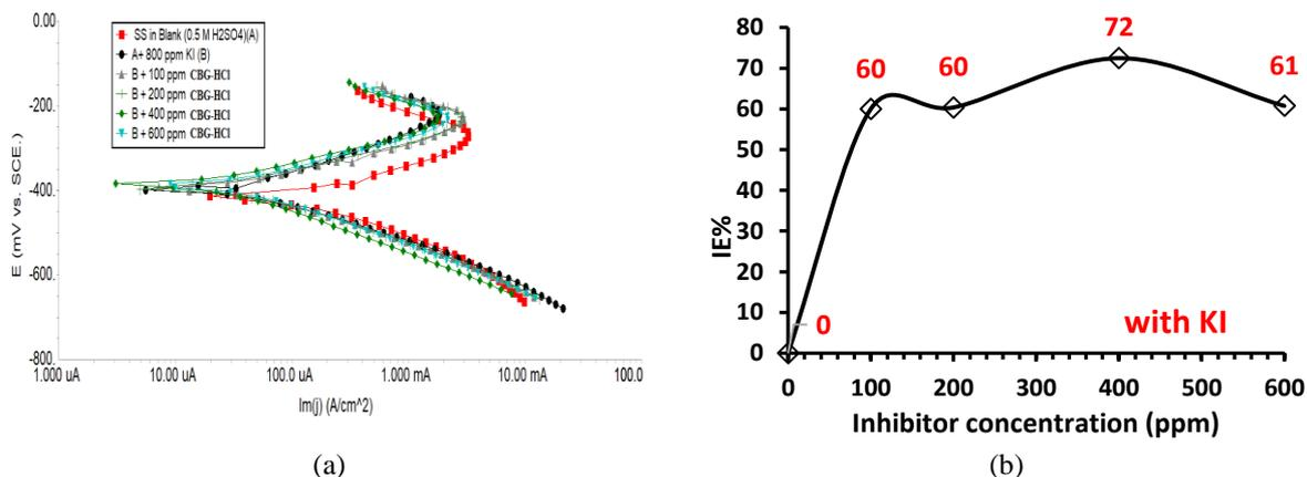
Fig. 6. (a) Potentiodynamic SS electrode plots were performed at different CBG-HCl concentrations together with 800 ppm KI in 0.5 M H<sub>2</sub>SO<sub>4</sub> solution. Rate of scan = 5 mV/s. (b) The average IE% obtained using EIS and potentiodynamic experiments conducted at 100, 200, 400 and 600 ppm of CBG-HCl concentration and together with 800 ppm KI on SS in 0.5 M H<sub>2</sub>SO<sub>4</sub> solution.
