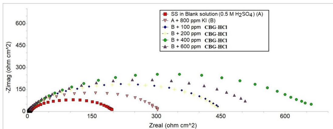
Fig. 3. Nyquist SS plot reported for the synergistic effect of 800 ppm of KI at different CBG-HCl concentrations in 0.5 M  $H_2SO_4$  at 298 K.
