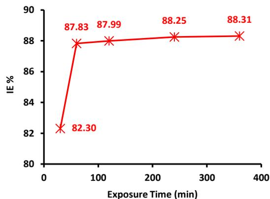
Fig. 8. EIS inhibition performance of a stainless-steel electrode immersed in a 0.5 M H<sub>2</sub>SO<sub>4</sub> solution in the presence of 400 ppm CBG-HCl and 800 ppm KI at different exposure time.
