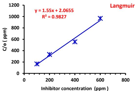
Fig. 7. Langmuir isothermal model plot for CBG-HCl inhibitor on the surface of stainless-steel alloy in acidic media.
