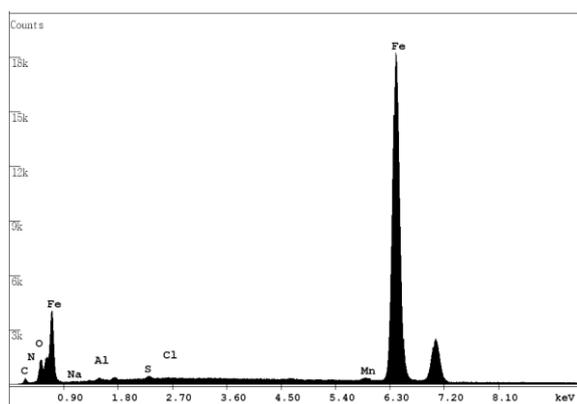
Fig. 9. EDX spectra obtained for stainless steel after 22 hours in 0.5 M H<sub>2</sub>SO<sub>4</sub> containing 400 ppm CBG-HCl and 800 ppm KI.
