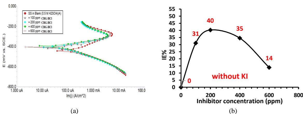
Fig. 5. (a) Stainless steel electrode potentiodynamic plots were reported at different CBG-HCl concentrations in a  $0.5 \text{ M H}_2\text{SO}_4$  solution. Rate of scan =  $5 \text{ mV/s}$ , (b) The average IE% values of CBG-HCl on SS in  $0.5 \text{ M H}_2\text{SO}_4$  solution. The data represent the average IE% values obtained using EIS and potentiodynamic experiments conducted at 100, 200, 400 and 600 ppm concentration of CBG-HCl.
