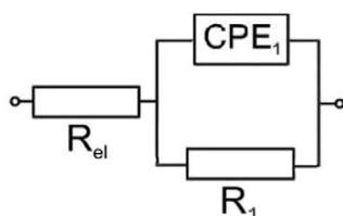
Fig. 4. EEC model was applied to represent EIS information collected on stainless steel electrodes immersed in 0-containing electrolytes and different inhibitor concentrations. Where, respectively,  $R_{el}$ ,  $R_1$  and CPE1 reflect solution resistance, polarization resistance, and double-layer capacitance.
