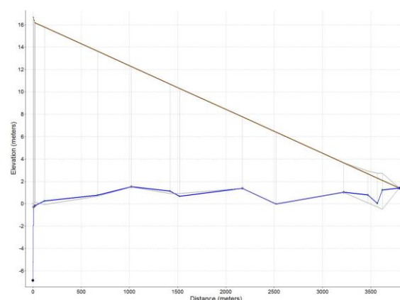
Figure (6) Hydraulic gradient for the pipeline at steady state in relative to pipeline profile after protection
