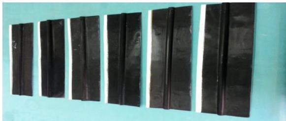
Figure 3 Preparation of multi samples by 2nd anodization and colouring for installation of primarily model solar water heater
