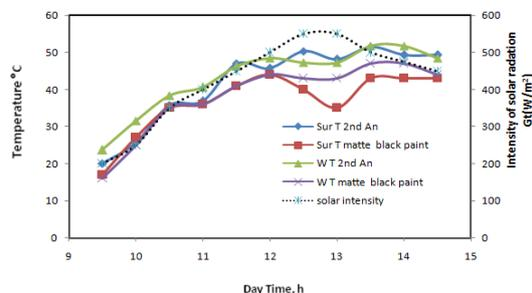
Figure 6 Variation of recorded temperatures (panel & outlet water) with intensity of solar radiation for both second anodized and matte black paint solar collectors without glass cover within day time.
