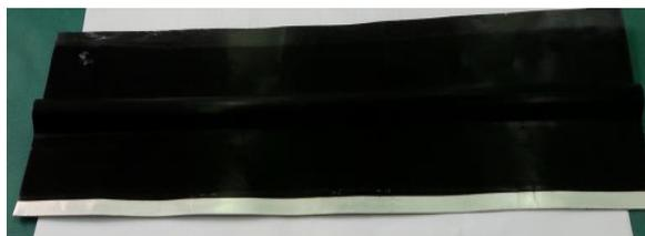
Figure 2 Sample of dimensions 40 x 15 cm after second anodization and electrolytic colouring
