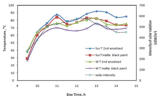
Figure 5 Variation of recorded temperatures (panel & outlet water) with intensity of solar radiation for both second anodized and matte black paint solar collectors with glass cover within day time.
