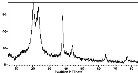
Fig. 8. XRD analysis of biosynthesize CuNPs nylon fabric .
