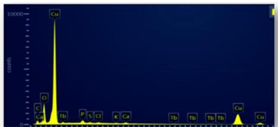
Fig. 5 : EDX image of biosynthesize CuNPs .
