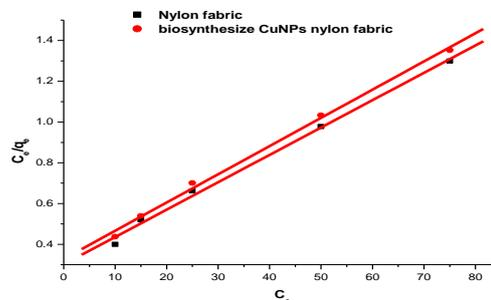
Fig .13: Langmuir adsorption isotherm of AB172 onto untreated and biosynthesize CuNPs nylon fabric at [LR 1:50, 90 °C].
