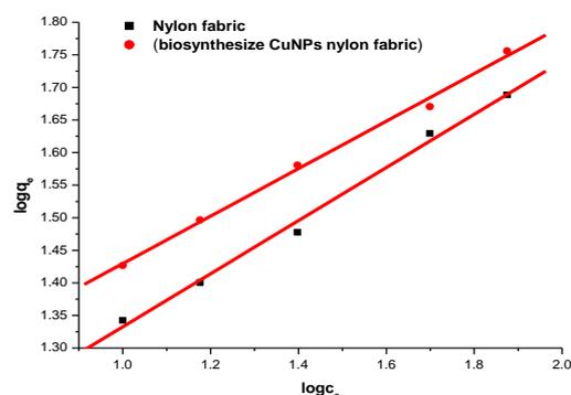
**Fig.14: Freundlich adsorption isotherm of AB172 onto untreated and biosynthesize CuNPs nylon fabric at [LR 1:50, 90 °C].**
