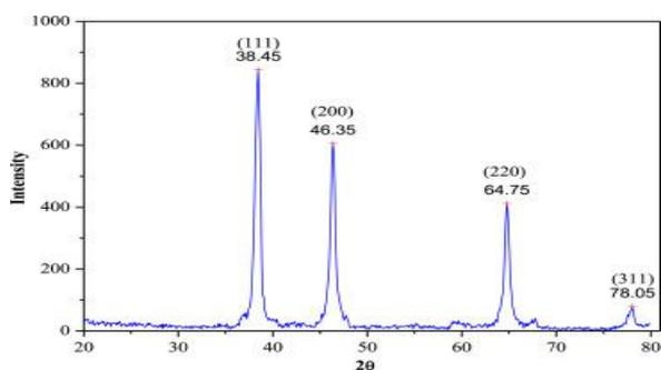
Fig. 7. XRD analysis of biosynthesize CuNPs .
