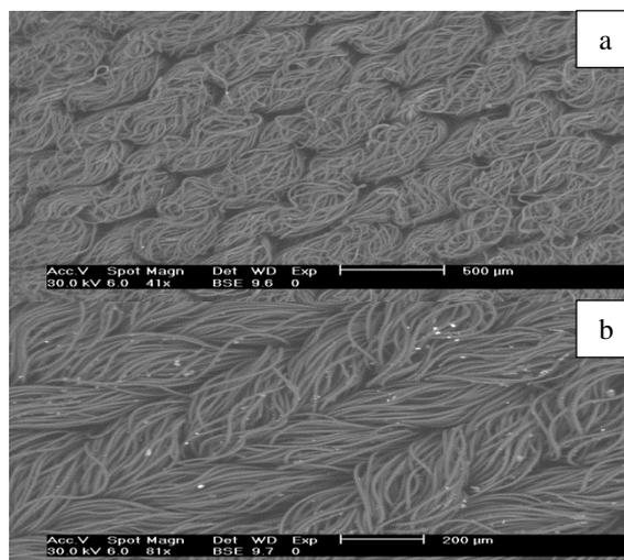
**Fig. 4 : SEM image of (a) nylon fabric (b) biosynthesize CuPNs nylon fabric**
