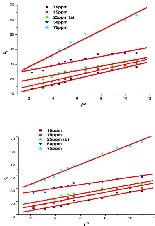
**Fig. 11:** Intra-particle diffusion kinetics of AB 172 into (a) untreated nylon fabrics (b) biosynthesize CuNPs nylon fabrics at various concentrations.[Dyeing recipe : LR 1:50, 90 °C].
