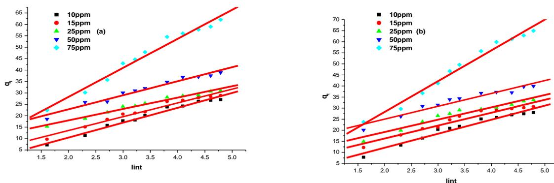
Fig.12 :Elovich diffusion kinetics plots of adsorbed AB 172 into (a) untreated nylon fabrics (b) biosynthesize CuNPs nylon fabrics at various concentrations.[Dyeing recipe : LR 1:50, 90 °C].
