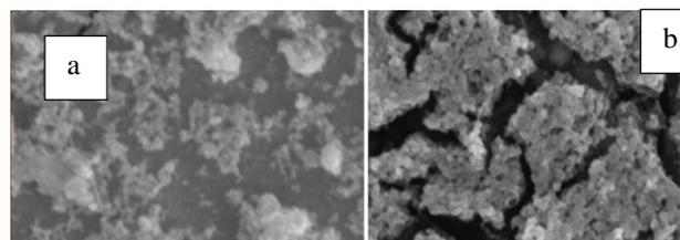
**Fig.3: SEM image of (a) biosynthesized copper nanoparticles, (b) high magnification**
