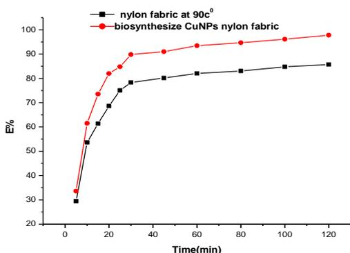
**Fig. 9: Time-Exhaustion isotherms of AB 172 dye adsorption onto untreated and pre-treated nylon fabric with green CuNPs . [dyeing recipe: LR 1:50, 25 ppm, 90°C].**
