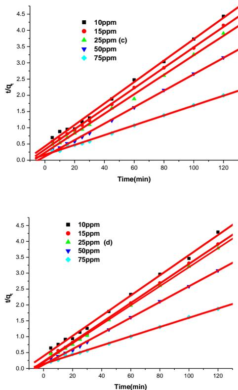
**Fig. 10 :** Kinetic plot for the adsorption of AB 172 onto nylon fabric at 90 °C .
