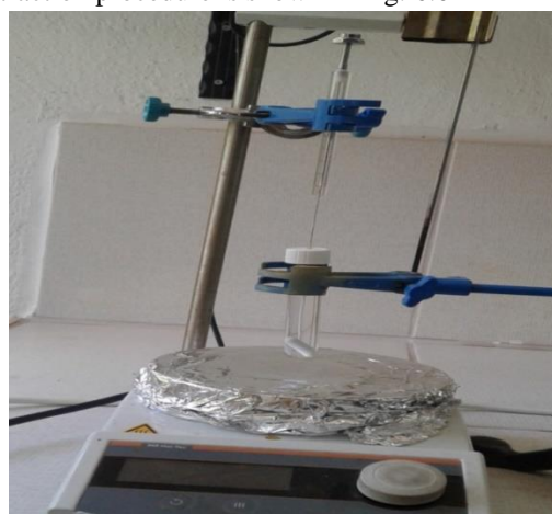
Fig. 6: Extraction process using hollow fiber membrane
