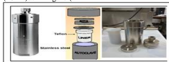
Fig. (1): Schematic of Autoclave Parr Reactor to a chives the hydrothermal method.
