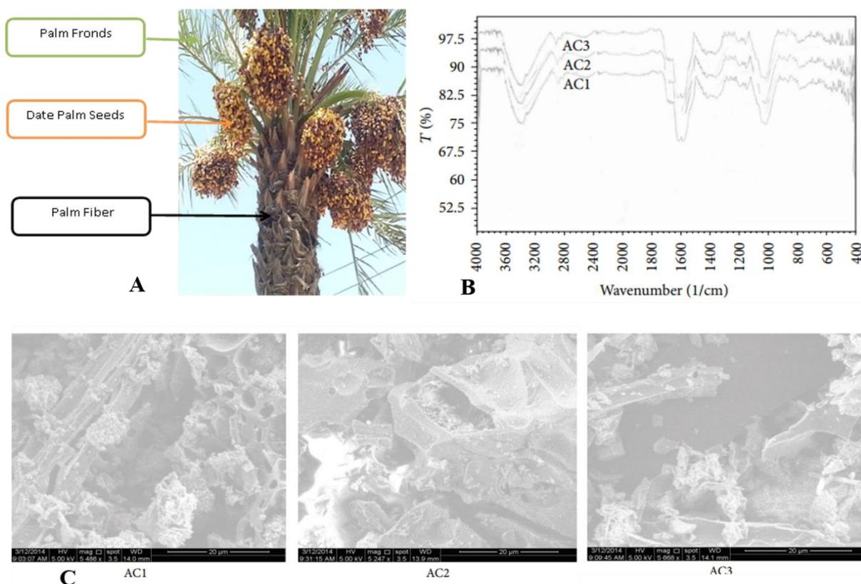
Fig. 8. (A) Diagrammatic representation of Iraqi Khestawy date palm structure. (B) FTIR spectra for AC1, AC2, and AC3 samples synthesized from Iraqi Khestawy date palm. (C) SEM images for the AC1, AC2, and AC3 samples synthesized from Iraqi Khestawy date palm [4].
