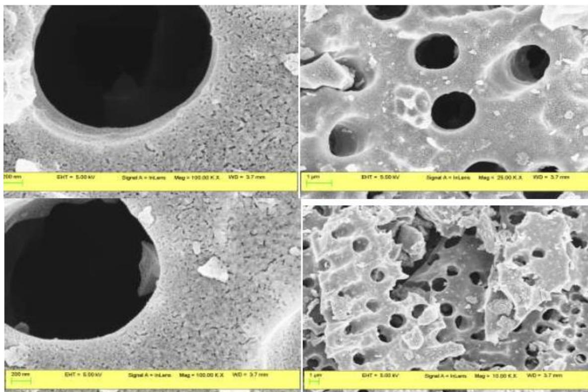
Fig. 5. SEM images of H<sub>2</sub>SO<sub>4</sub> impregnated coconut shell AC [23].
