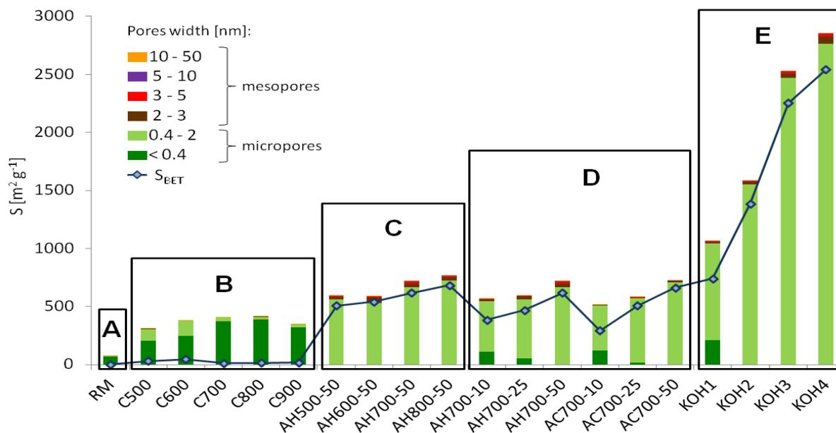
Fig. 3. Distribution of micro- and mesoporous surface area according to pore size and BET surface area in raw material (A), chars (B) and AC produced through steam activation at various temperatures (C), steam and  $\text{CO}_2$  activation to various burn-offs, (D) and chemical (potassium hydroxide) activation (E) [24].
