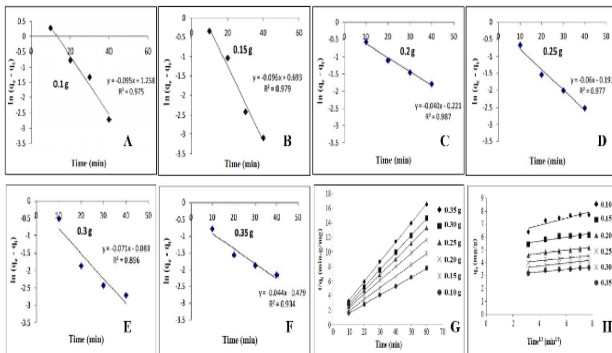
Fig. 10. Pseudo-first order kinetic model (A-F), pseudo-second order kinetic model (G), and intraparticle diffusion model (H) for the adsorption of disperse blue dye onto ZDSAC [58].
