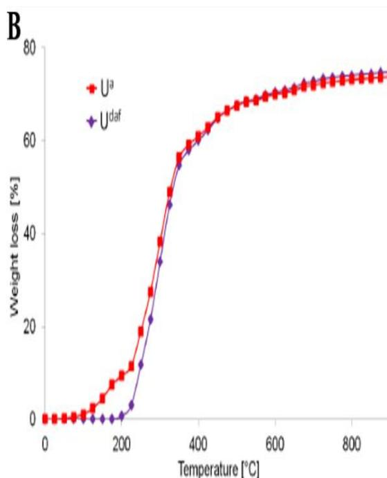
Fig. 1. (A) Giant knotweed pellets used as a raw material for AC preparation. (B) Thermogravimetric analysis of giant knotweed pellets in analytical state (U<sup>a</sup>) and dry ash-free state (U<sup>daf</sup>) [24].
