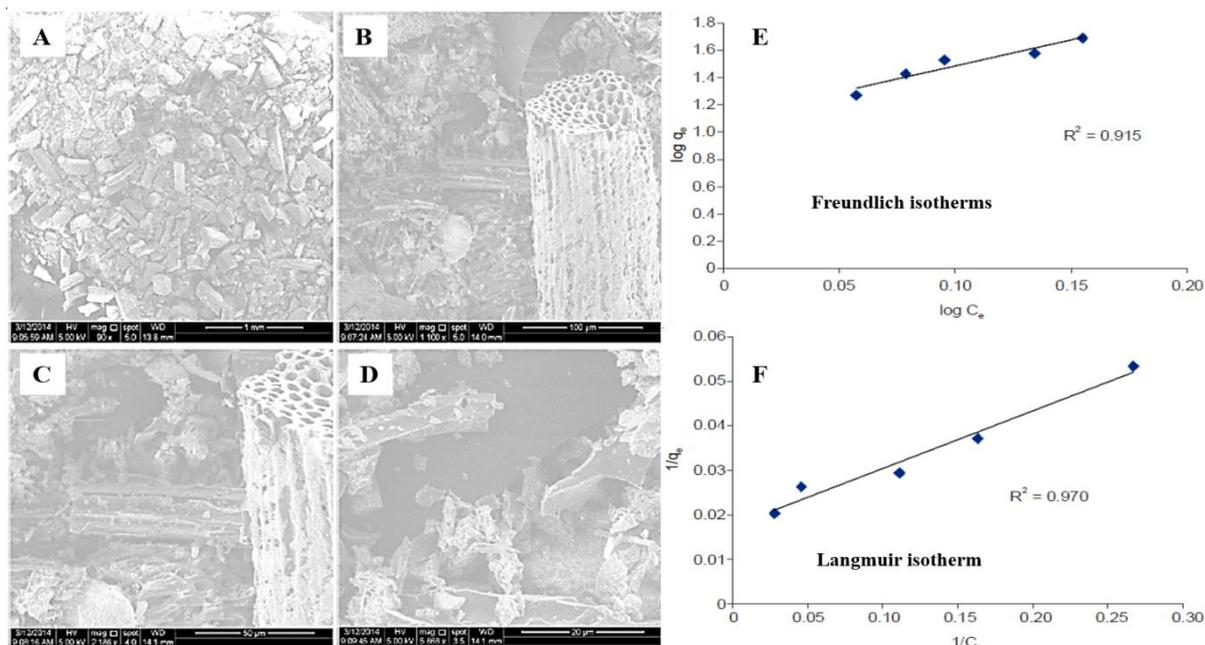
Fig. 7. SEM micrographs of carbon samples from Iraqi Palm fiber: 200 mesh (A, B, C and D at different magnifications). (E) The linear Freundlich adsorption isotherms for brilliant cresyl blue dye adsorption by the activated Iraqi palm fiber carbon. (F) The linear Langmuir adsorption isotherms for brilliant cresyl blue dye adsorption by the activated Iraqi palm fiber carbon [57].
