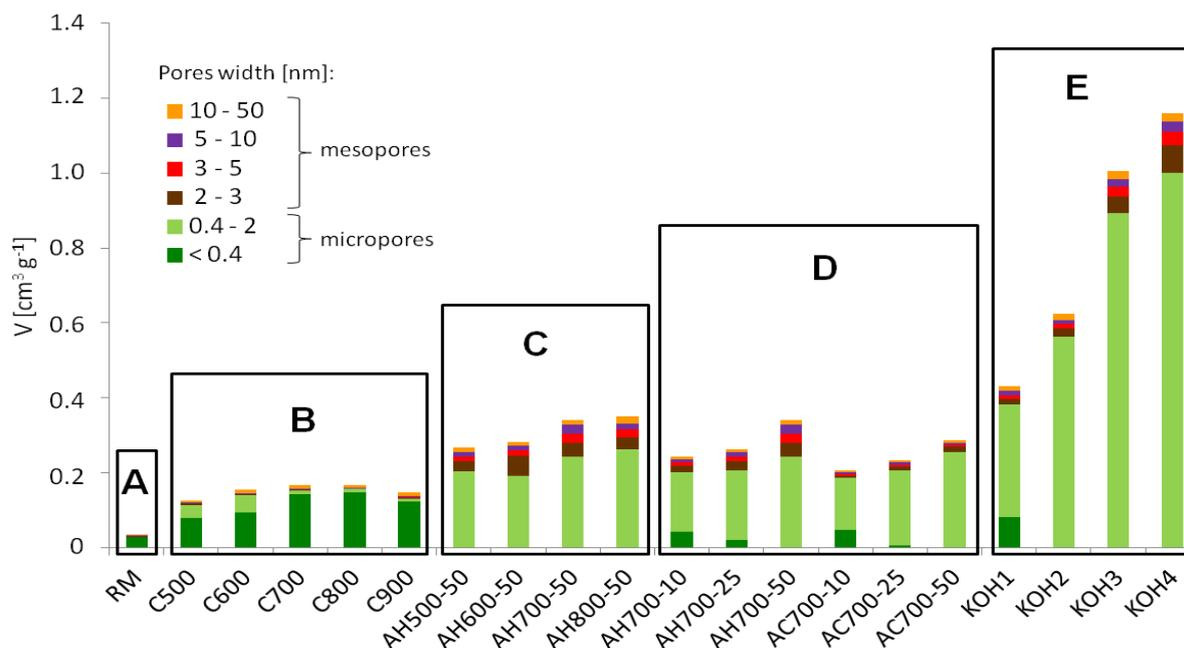
Fig. 2. Distribution of micro- and mesoporous volume according to pore size in raw material (A), chars (B) and AC got by steam activation at various temperatures (C), steam and  $\text{CO}_2$  activation to various burn-offs (D) and chemical (potassium hydroxide) activation (E) [24].
