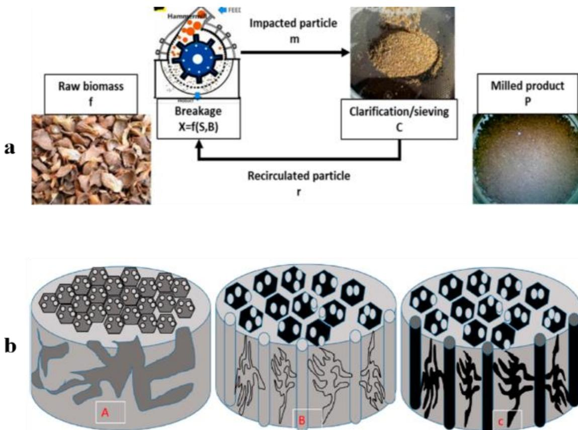
Fig. 4. (a) Hammer milling process for biomass. (b) Activation temperature's influence on AC pore development and morphology A: biomass structure; B: partially developed char structure; C: well-defined porous AC structure [2].
