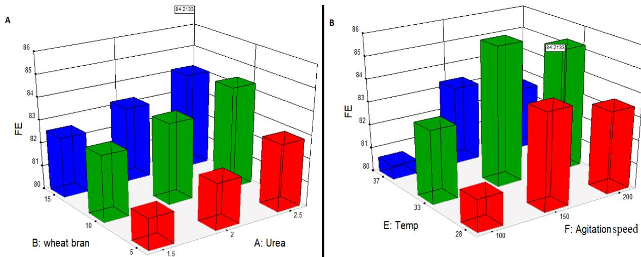
Fig. 3. (A) The interaction between urea and wheat bran and their effect on FE %, (B) The interaction between temperature and agitation speed and their effect on FE %.
