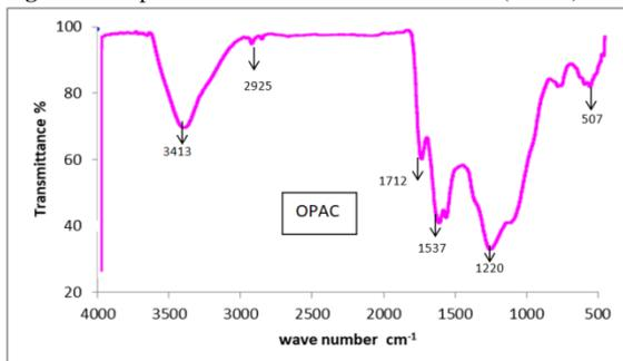
Fig. 2. FTIR spectrum of oxidized activated carbon (OPAC)
