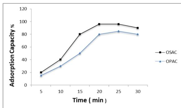
Fig. 4. Effect of contact time on adsorption capacity by OSAC and OPAC
