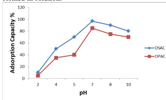
Fig. 6. Effect of PH on adsorption capacity by OSAC and OPAC
