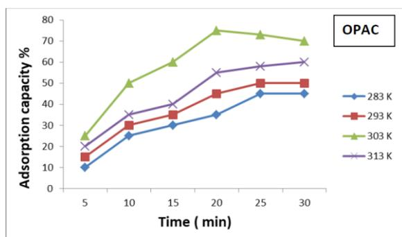
Fig. 8. Effect of temperature on adsorption capacity by OPAC
