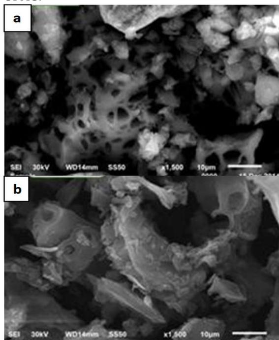
Fig. 3. a: SEM photographs of OSAC b: SEM photographs of OPAC
