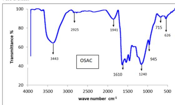
Fig. 1. FTIR spectrum of oxidized activated carbon (OSAC)
