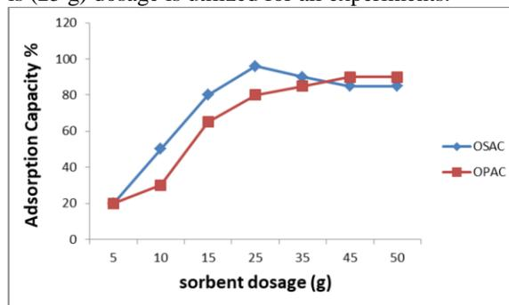
Fig. 5. Effect of sorbent dosage on adsorption capacity of OSAC and OPAC
