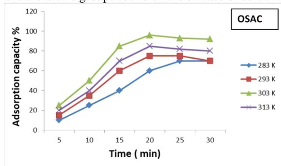
Fig. 7. Effect of temperature on adsorption capacity by OSAC
