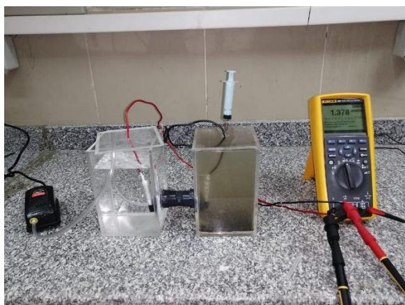
Fig. 1: A photograph showing one of the installed MFCs.
