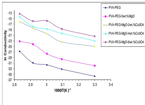
**Fig. 4.** In conductivity versus  $(1000/T)$  of (PVA-PEG) blend and its composite with MgO and different wt.% of  $\text{Co}_3\text{O}_4$  films.
