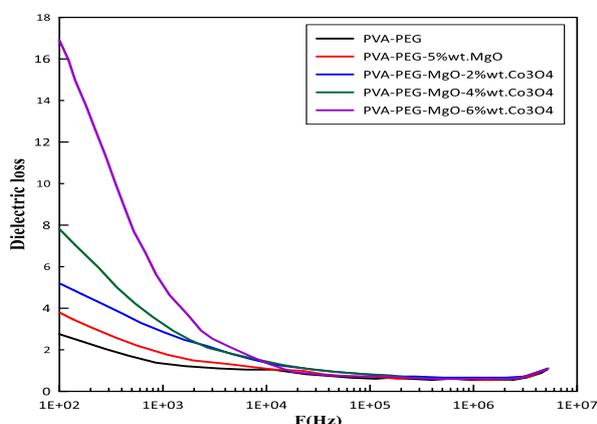
Fig. 7. Variation of dielectric loss of (PVA-PEG) blend and its composite with MgO and different wt.% of  $\text{Co}_3\text{O}_4$  films versus frequency at RT
