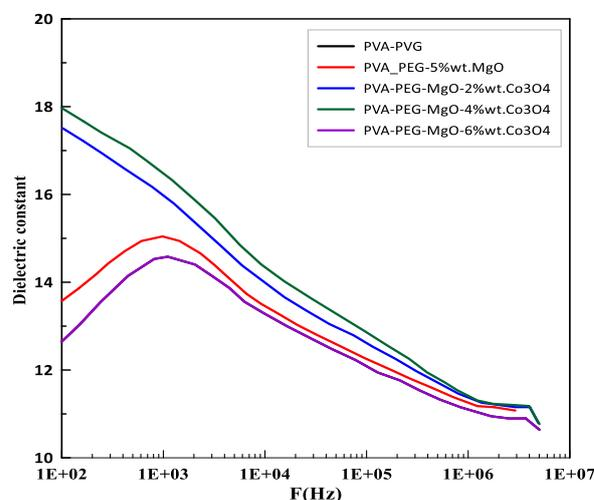
**Fig.5.** Variation of dielectric constant of (PVA-PEG) blend and its composite with MgO and different wt.% of  $\text{Co}_3\text{O}_4$  films versus frequency at RT
