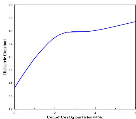
Fig.6. Effect of  $\text{Co}_3\text{O}_4$  particles concentrations on dielectric constant of (PVA-PEG) –in the case of constant MgO at 100Hz
