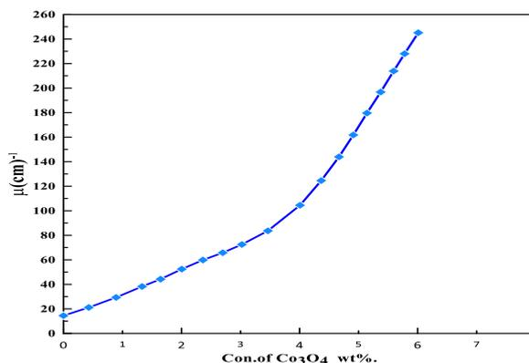
**Fig. 12.** The attenuation coefficients varied with gamma radiation for (PVA-PEG-5wt.%MgO) composite with different concentrations of  $\text{Co}_3\text{O}_4$  particles.
