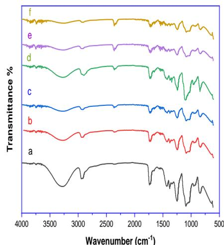
**Fig.1.** FTIR spectra of: a. PVA, b. (PVA-PEG) blend, c. (PVA-PEG-5wt.% MgO), d. (PVA-PEG-MgO-2wt.%  $\text{Co}_3\text{O}_4$ ), e. (PVA-PEG-MgO-4wt.%  $\text{Co}_3\text{O}_4$ ), and f. (PVA-PEG-MgO-6wt.%  $\text{Co}_3\text{O}_4$ ) composite films.
