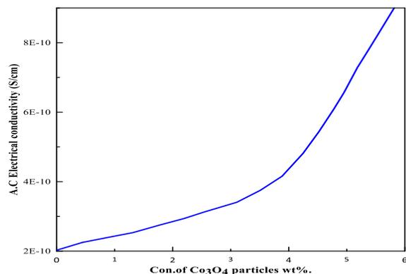
**Fig.10.** Effect of  $\text{Co}_3\text{O}_4$  particles concentrations on the electrical conductivity of A.C. for (PVA-PEG) in the case of constant MgO at 100Hz.
