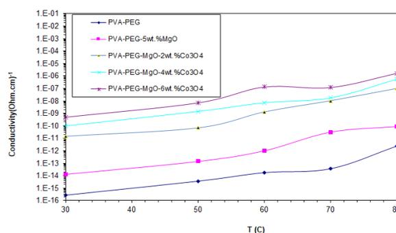
**Fig. 3.** The conductivity of D.C. for (PVA-PEG) blend and its composite with MgO and different wt.% of  $\text{Co}_3\text{O}_4$  films with temperature.
