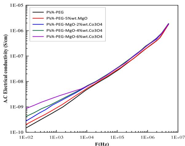
Fig.9. The electrical conductivity of A.C for (PVA-PEG) poly-blend and its composite with MgO and different wt.% of  $\text{Co}_3\text{O}_4$  films versus frequency at RT
