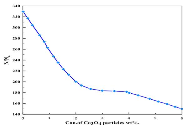
**Fig.11.** Variation of  $(N/N_0)$  for (PVA-PEG-5wt.%MgO) composite with different concentrations of  $\text{Co}_3\text{O}_4$  particles.
