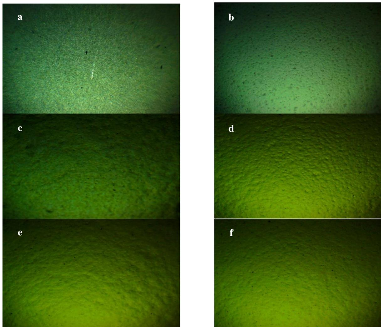
**Fig. 2:** Optical microscopy at (40X) of: a. (PVA), b. (PVA-PEG) blend, c. (PVA-PEG-5wt.% MgO), d. (PVA-PEG-MgO-2wt.%  $\text{Co}_3\text{O}_4$ ), e. (PVA-PEG-MgO-4wt.%  $\text{Co}_3\text{O}_4$ ), and f. (PVA-PEG-MgO-6wt.%  $\text{Co}_3\text{O}_4$ ) composite films.
