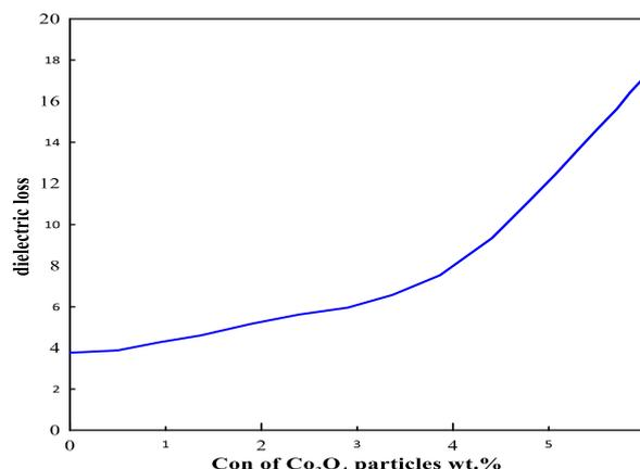
Fig.8. Effect of  $\text{Co}_3\text{O}_4$  particles concentrations on dielectric loss of (PVA-PEG) in the case of constant MgO at 100Hz.
