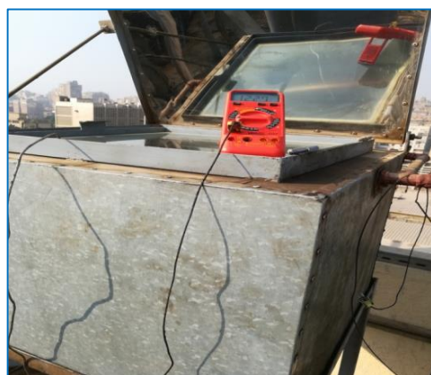
Fig 6: A photographic view of the Thermocouples inside/outside the baking unit.
