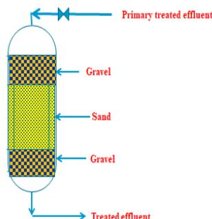
Fig.1. Schematic diagram of sand filter column
