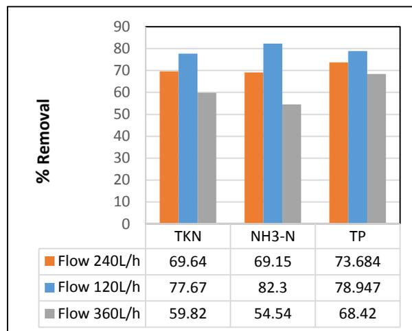
Fig.6. Effect of flow rates on nutrients removal
