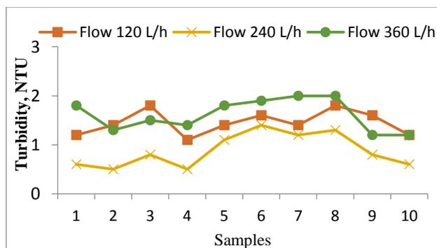
Fig.3. Effect of flow rate on Turbidity
