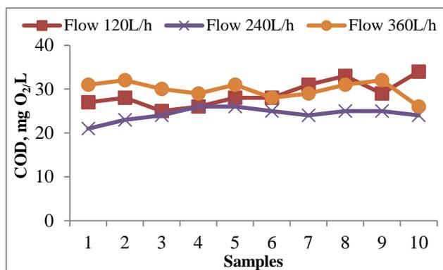
Fig. 5. Effect of flow rate on COD
