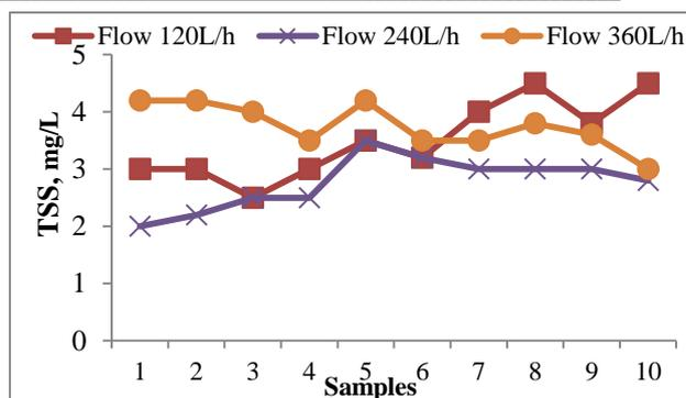
Fig. 4. Effect of flow rate on TSS
