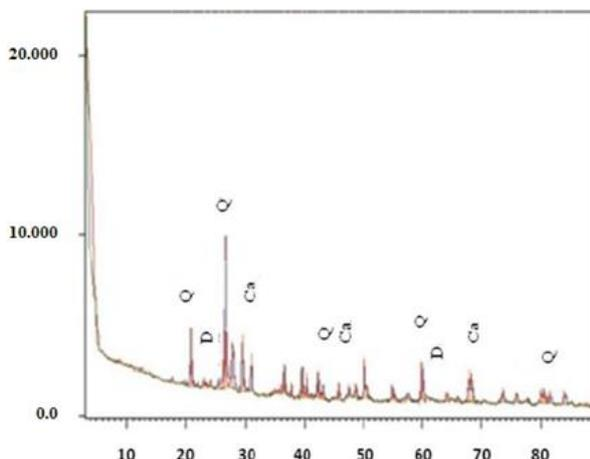
Fig.2. X-ray Diffractogram of the used sand, (Q: quartz; D: Dolomite; Ca: Calcite)
