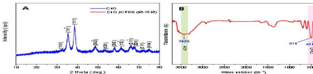
Figure 1. (A) XRD patterns of CuO-NPs;
