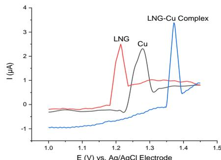
**Fig.2:** Square wave voltammograms of Cu ( $5.32 \text{ μg mL}^{-1}$ ), LNG ( $94.50 \text{ ng mL}^{-1}$ ), and LNG-Cu complex ( $47.25 \text{ ng mL}^{-1}$ ) on Cu-PGE
