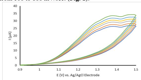
**Fig. 1:** Typical cyclic voltammograms for  $94.50 \text{ ng mL}^{-1}$  LNG of LNG-Cu complex using Cu-PGE at scan rate values (0.1, 0.2, 0.3, 0.4, 0.5, and 0.6 V) of 60 s accumulation time
