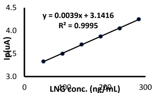
**Fig.7:** Calibration curve of LNG-Cu complex at six concentration (a)47.25, (b)94.51, (c)141.76, (d)189.02, (e)236.27, and (f)283.52 ng ml<sup>-1</sup> of LNG in LNG-Cu complex on electrode surface at IP +0.9, BR Buffer pH 4.5 0.04M, and 430 s accumulation time.
