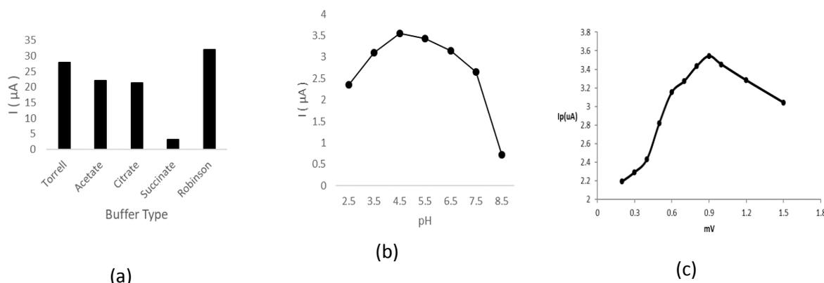
**Fig.4:** (a) Effect of type of buffer, (b)Effect of pH, and (c) Effect of buffer concentration in presence 94.51 ng ml<sup>-1</sup> of LNG in LNG-Cu complex on electrode surface at 60 s accumulation time
