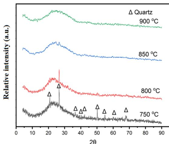
**Figure 3.** XRD patterns of glass / ceramic composite sintered at different temperatures.
