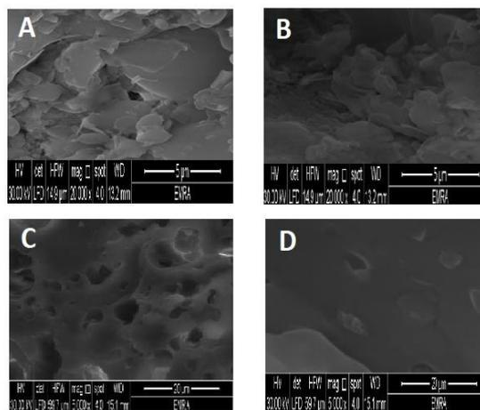
**Figure 2.** SEM micrographs of glass / ceramic composite prepared at different sintering temperatures (GC from A to D).
