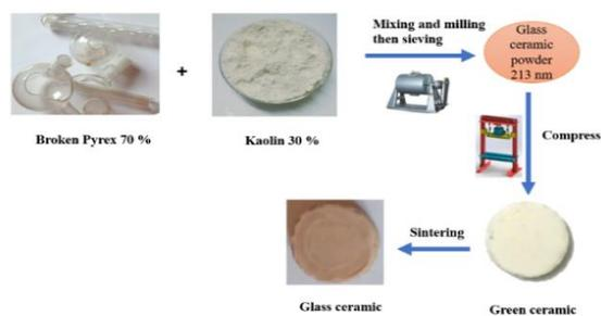
**Figure 1.** Schematic diagram for the preparation of borosilicate glass / ceramic composite.
