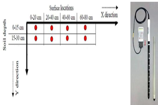
Locations of soil moisture content before and after irrigation and using profile probe for measuring
