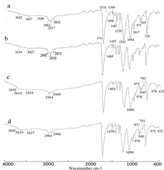
**Figure 4:** FTIR spectra of (a) untreated PET, (b) treated PET/8%NaOH, (c) PET/ 1%  $\text{SiO}_2$  NPs and (d) PFT/ 1.5%  $\text{SiO}_2$  NPs
