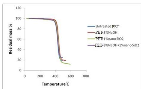
**Figure 5:** TGA diagram of PET, PET/8% NaOH, PET/1% SiO<sub>2</sub>NPs and PET/8%NaOH/ 1% SiO<sub>2</sub>NPs
