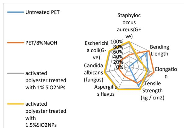
**Figure 6:** Radar chart of untreated and treated polyester fabrics with SiO<sub>2</sub>NPs
