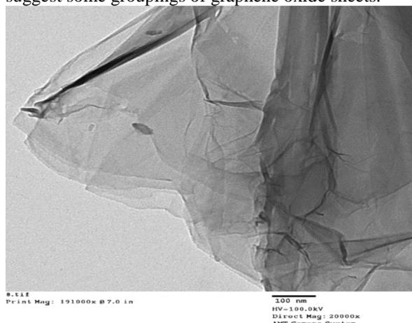
**Figure 4: HRTEM of the glycine-graphene oxide material.**
