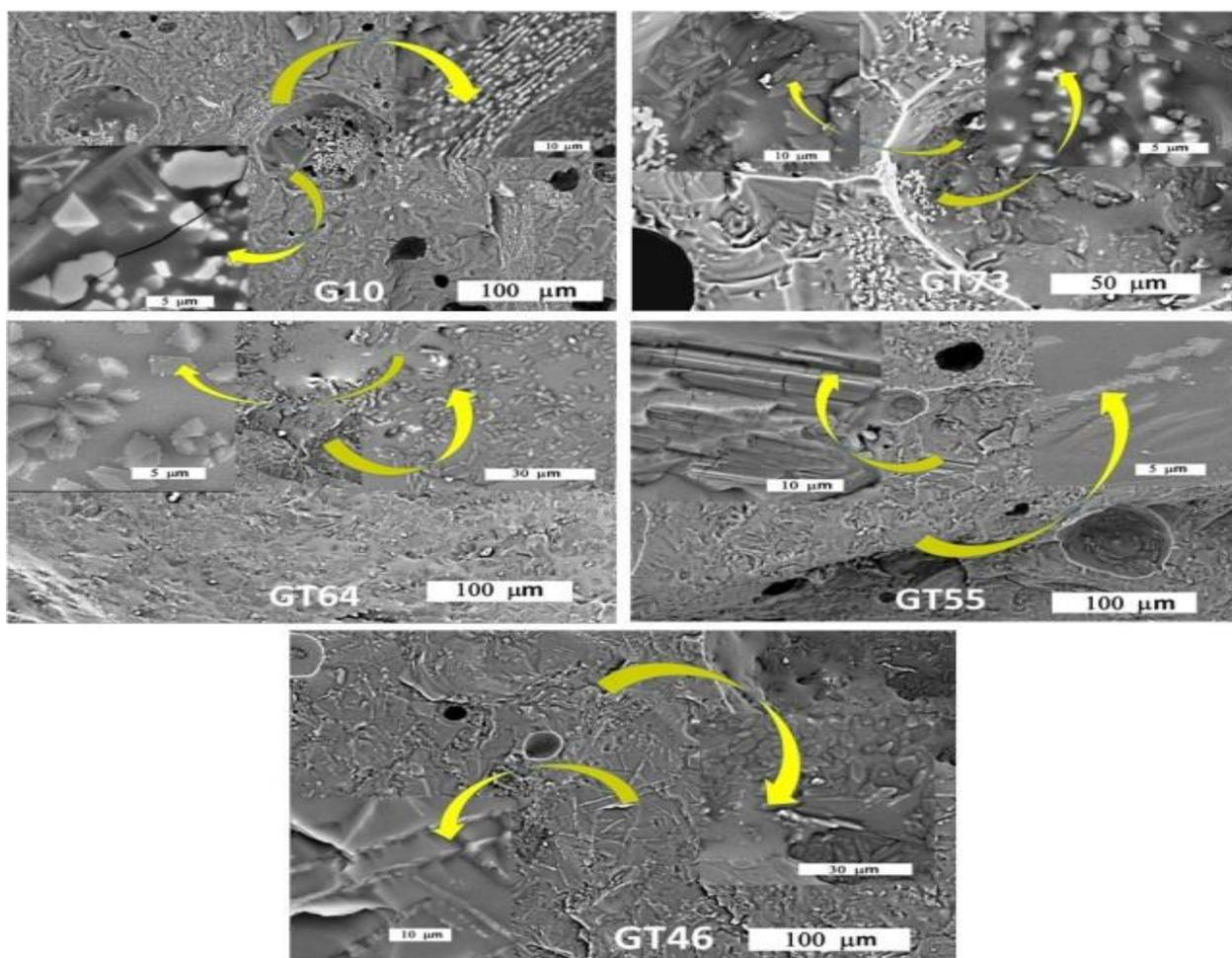
Fig. 7. SEM micrographs of G10, GT73, GT64, GT55 and GT46 samples sintered at different temperatures
