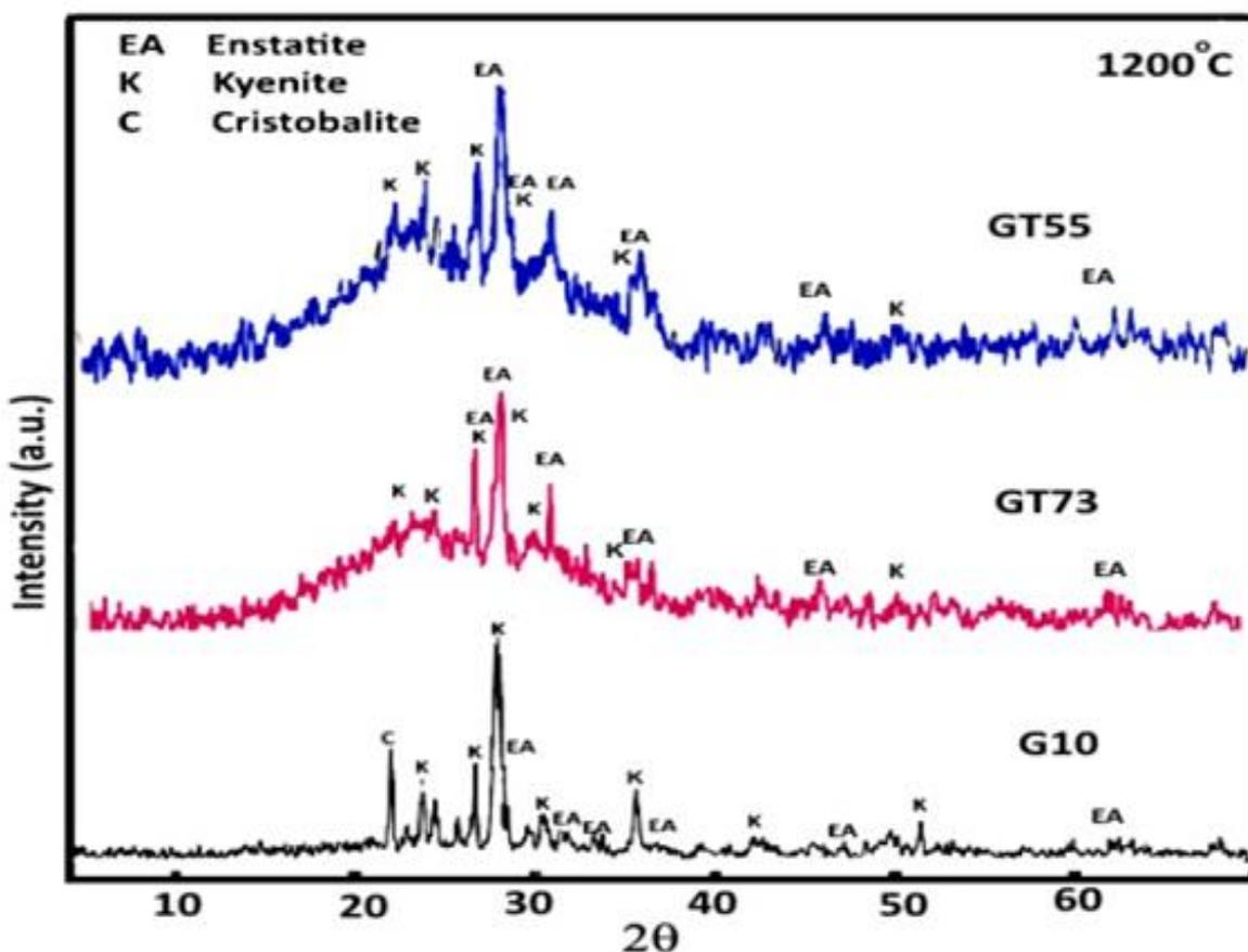
Fig. 4. X ray diffraction patterns of G10, GT73 and GT55 sintered at 1200 °C for 2h.
