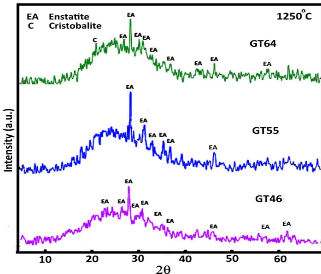
Fig. 5. X ray diffraction patterns of GT46, GT55 and GT64 sintered at 1250 °C for 2h.
