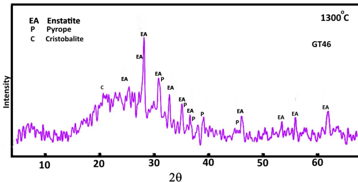
Fig. 6. X ray diffraction patterns of GT46 sintered at 1300 °C for 2h.
