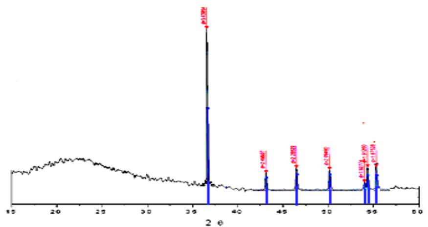
Fig. 3. XRD- of composite of silica gel with calcium carbonate .
