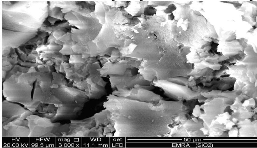
Fig. 5. SEM-image of pure silica calcined at 550°C.
