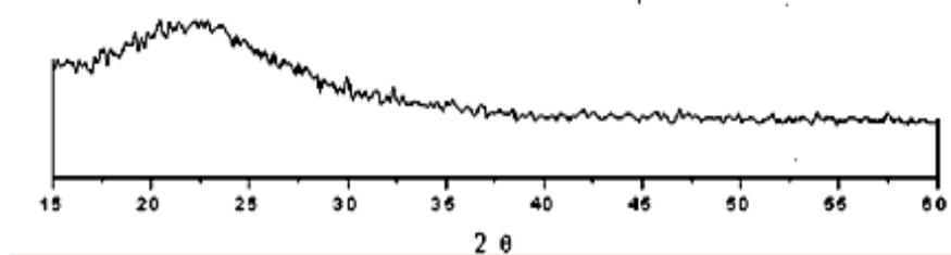
Fig. 2. XRD- of pure silica gel.
