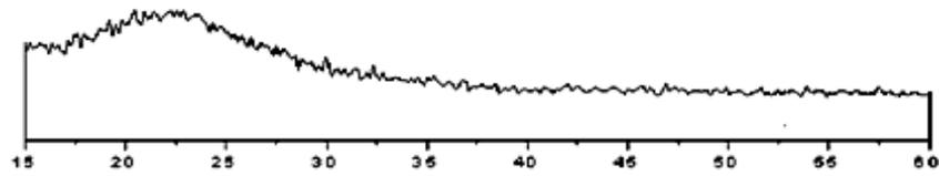
Fig. 4. XRD- of composite of silica gel after removal of calcium carbonate.
