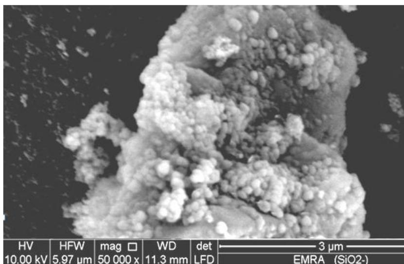
Fig. 7. SEM-image of silica nanoparticles treated with HCl and calcined at 550°C.
