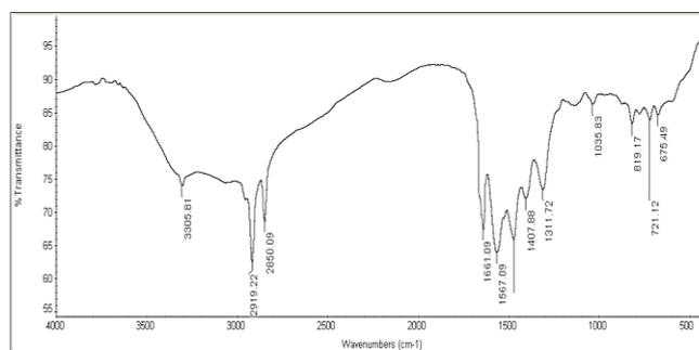
**Figure 1.** FTIR spectra of iphI (poly-3-(dodecylthio)-N-hexadecylacrylamide) ionophores.
