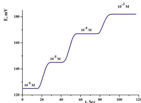
**Figure 3.** Calibration curve for Cr(III) ion using modified carbon paste electrode (electrode IV).
