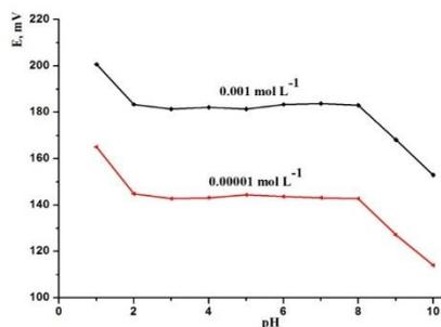
**Figure 6.** Effect of pH of the test solution on the potential readings of modified CPE sensor (electrode IV).
