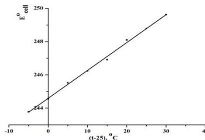
**Figure 7.** Variation of the cell e.m.f. with the temperature for the modified CPE sensor (electrode IV).
