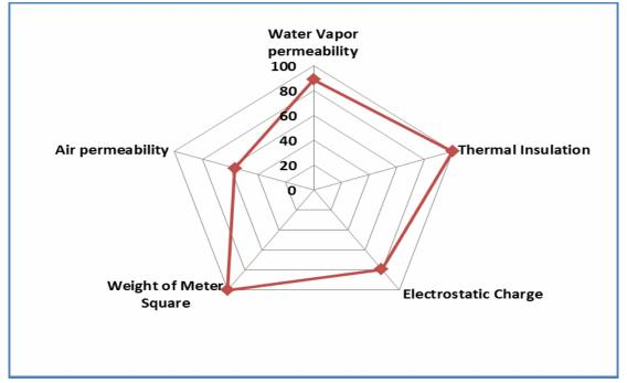
Fig. 5. The total quality factor for the best samples No. 9 with an perfect area (424.52) and the quality factor (84.90) with Genjar Concentration (100 %) and number of layers (3)
