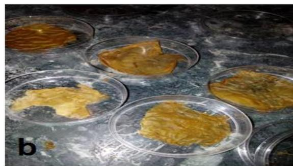
**Figure 5.** Fiber Produced after the Addition of glutaraldehyde
