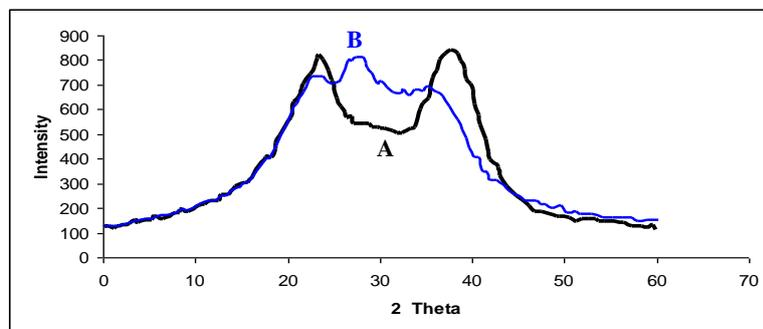
**Fig. 1.** XRD patterns for A) Pure PA6 and B) PA6/CaO nanocomposite.
