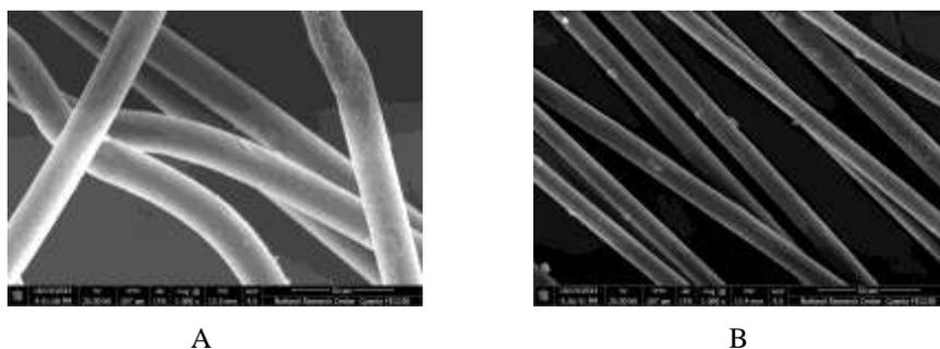
Fig. 5. SEM images for A) Pure PA6 and B) PA6/CaO nanocomposite.
