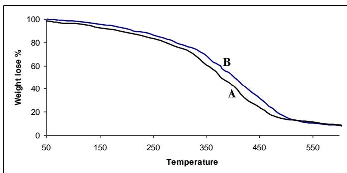
**Fig. 3. TGA Thermograms for A) Pure PA6 and B) PA6/CaO nanocomposite.**
