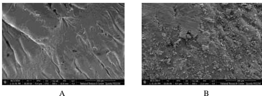
**Fig. 2.** SEM image for A) Pure PA6 and B) PA6/CaO nanocomposite.
