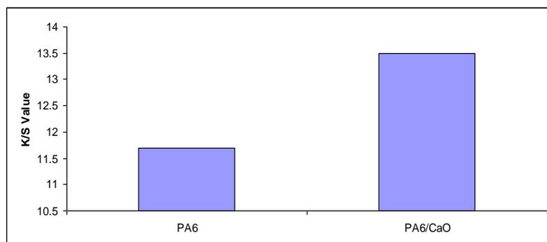
**Fig. 6.** Effect of disperse dyes on the colour strength of polyamide fibers.
