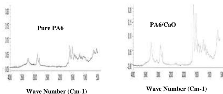
Fig. 4. FT-IR for A) Pure PA6 and B) PA6/CaO nanocomposite.
