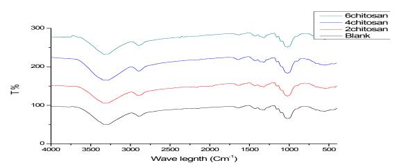
Fig(3a). FT-IR of the treated Shibeka fabrics treated with different chitosan concentration.
