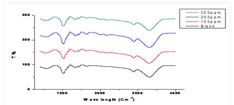
Fig (3b). FT-IR of the treated Shibeka fabrics treated with different silver concentration .
