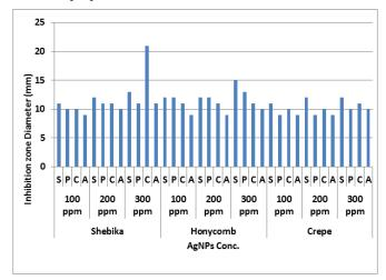
\*NB : Inhibition zone diameter of untreated fabrics equal zero mm Fig. 2. Effect of AgNPs concentrations on antimicrobial properties of treated fabrics.
