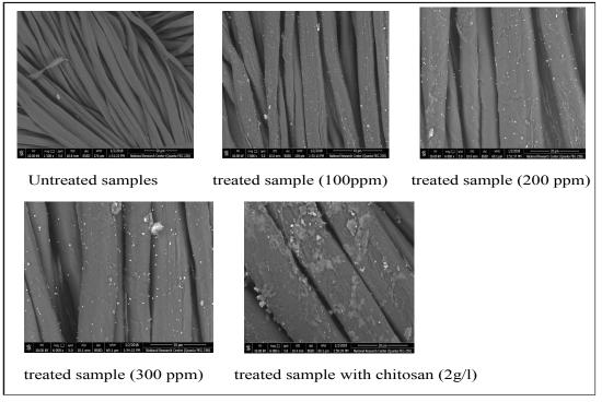
Fig.4. SEM images of the treated Shibeka fabrics with different AgNPs concentration and chitosan (2g/1).
