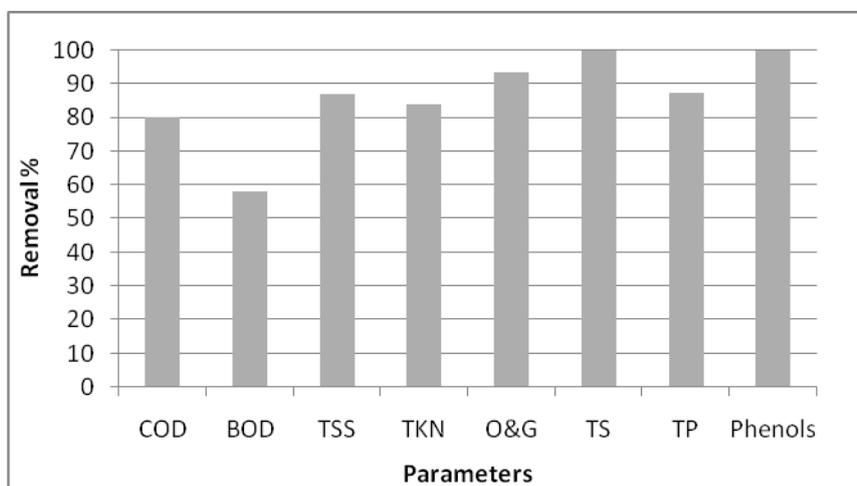
Fig. 5. Efficiency of Fenton process on the treatment of gas processing wastewater at optimum operating conditions.
