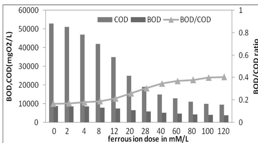
Fig. 3. Effect of different  $\text{Fe}^{2+}$  doses on the COD removal and BOD/COD ratio.
