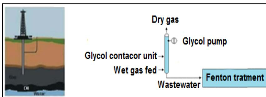
Fig. 1. Schematic diagram of the natural gas wastewater sources and the proposed treatment method.
