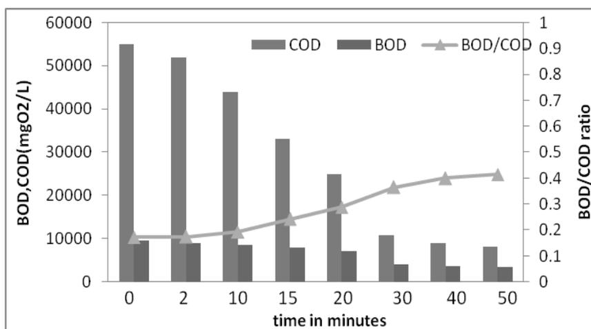
**Fig. 4.** Effect of reaction times on the removal of COD and BOD/COD ratio.
