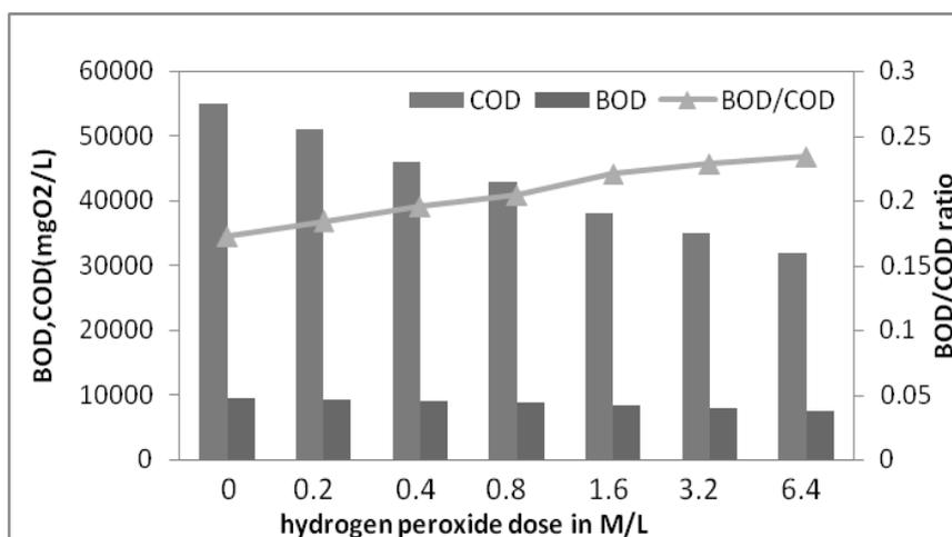
Fig. 2. Effect of different hydrogen peroxide doses on COD removal and BOD/COD ratio.
