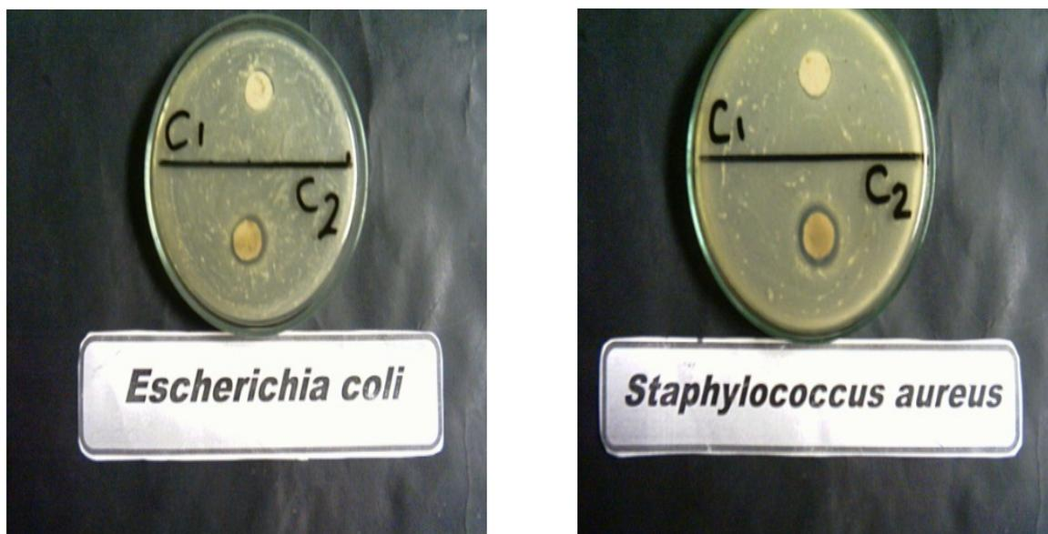
Fig.7. The antibacterial activity tests for C1 (CNP coating) and C2 (CNP+SNP coating) toward *E. coli* and *S. aureus* bacteria.
