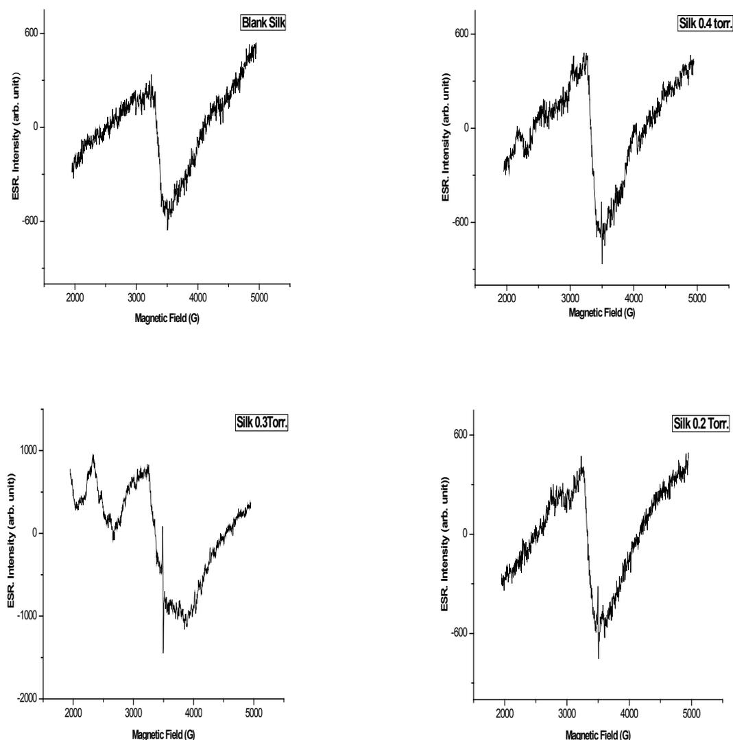
**Fig. 5.** The change in ESR intensity of plasma untreated and treated silk samples at different plasma pressure.
