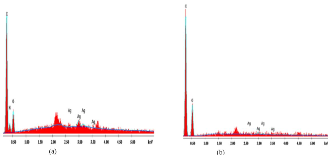
Fig. 11 (a, b). EDX spectrum of silver nano-particles treated samples.
