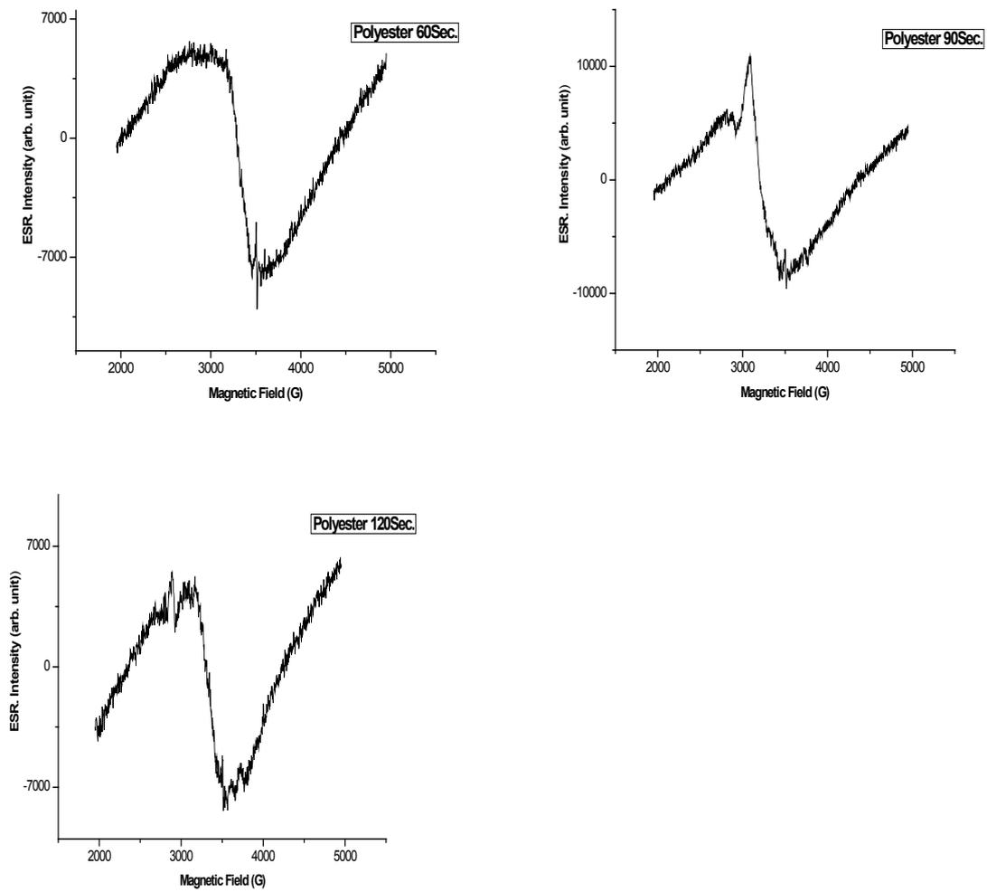
Fig. 2. The change in ESR Intensity of plasma untreated and treated polyester samples at different exposure times
