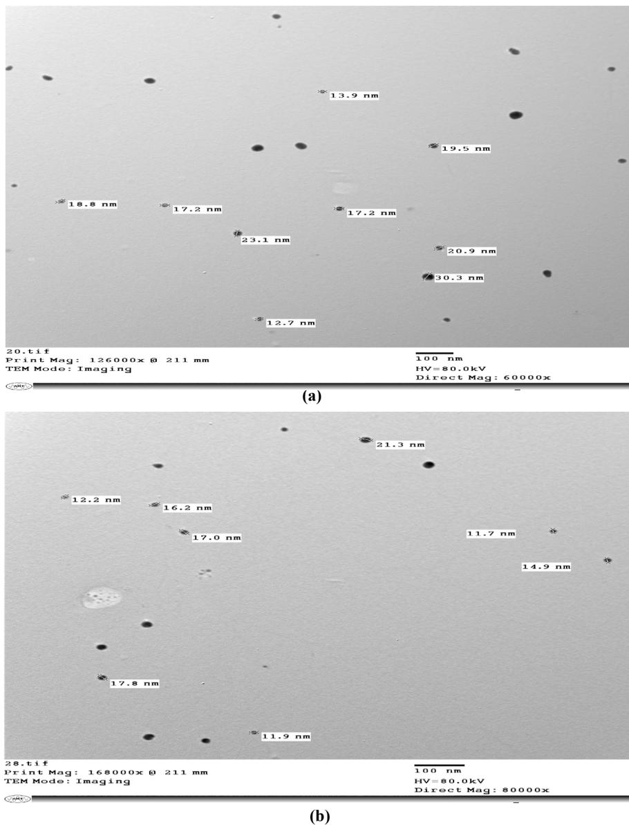
Fig. 8 (a,b). TEM of synthesized silver nano-particles.
