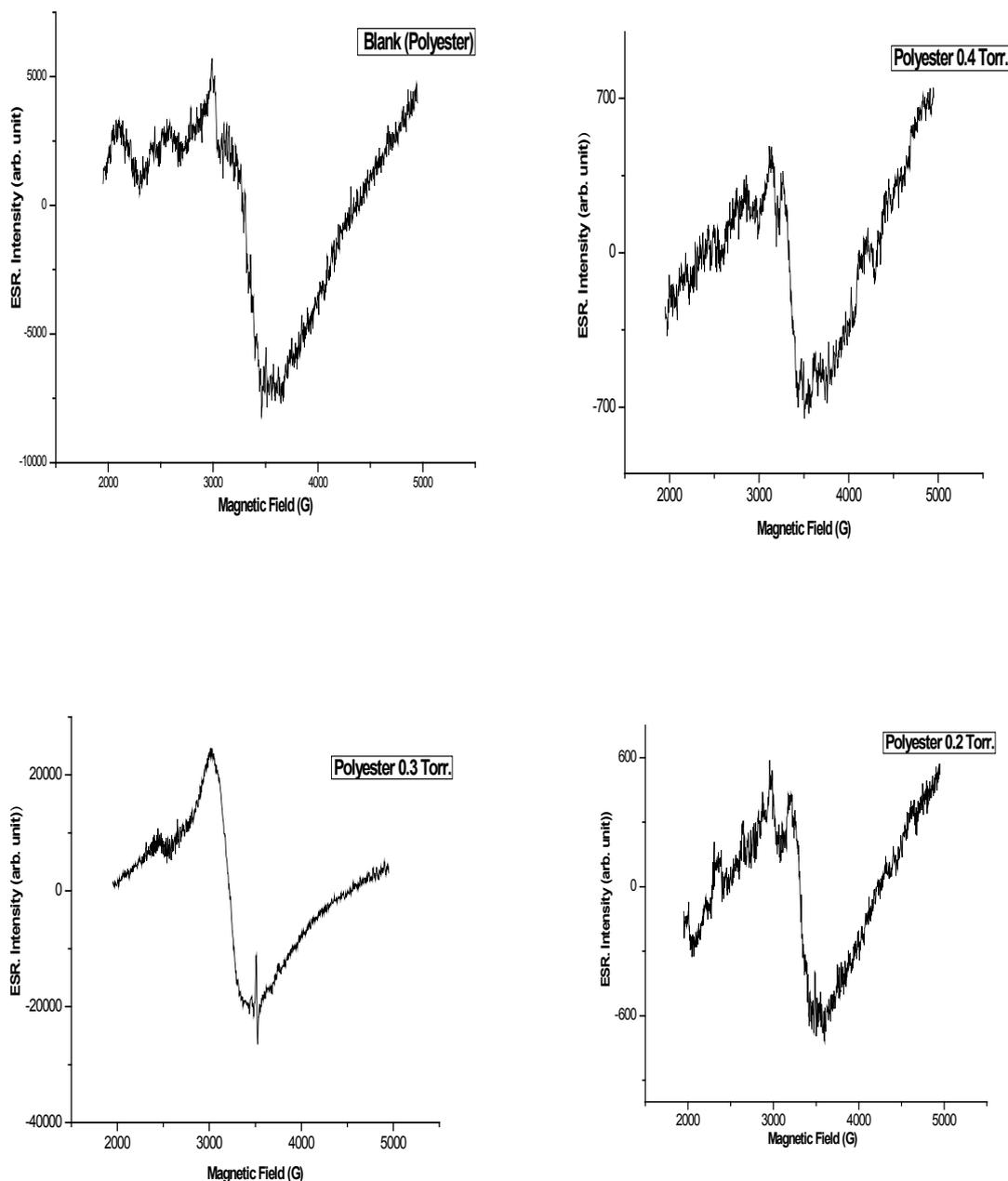
Fig. 4. The change in ESR intensity of plasma untreated and treated polyester samples at different plasma pressure.
