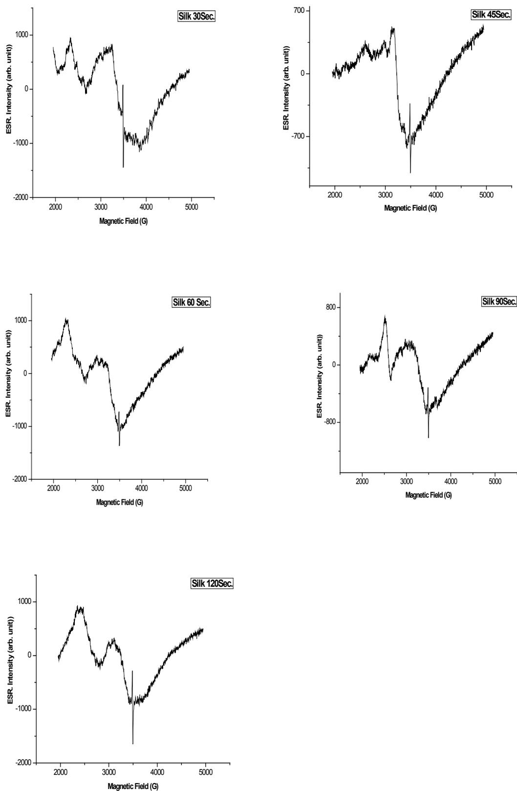
Fig. 3. The change in ESR Intensity of plasma untreated and treated silk samples at different exposure times.
