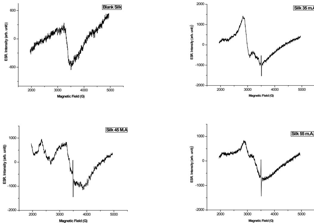
Fig. 7. The change in ESR intensity of plasma untreated and treated silk samples at different plasma current.
