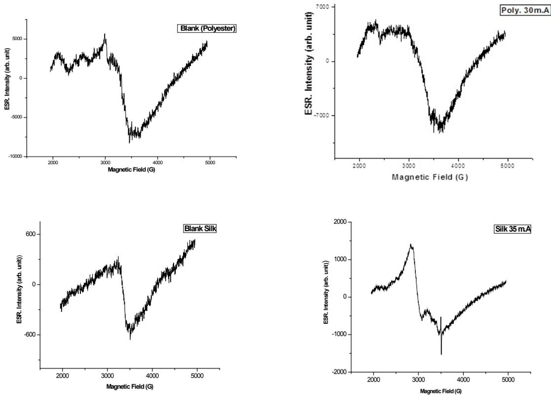
Fig. 6. The change in ESR Intensity of plasma untreated and treated polyester samples at different plasma current.
