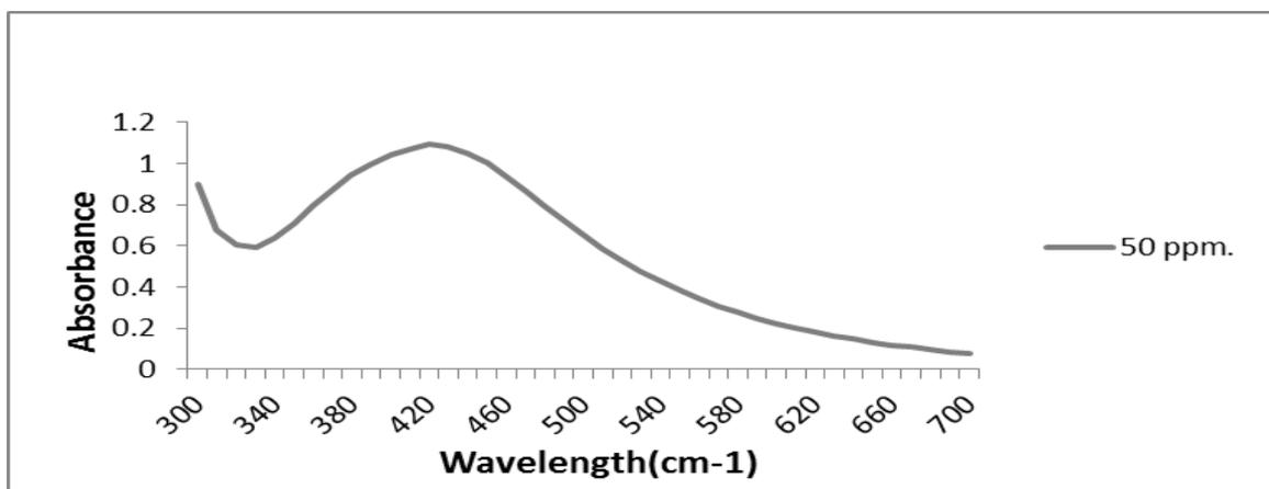
Fig. 9. UV-Vis spectra of 50ppm. Nano-silver colloidal solution.
