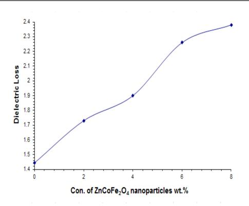
Fig. 4. The variation of dielectric loss with the concentration of filler at 100Hz.
