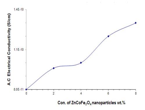
Fig. 6. The variation of electrical conductivity of (PS-Cr<sub>2</sub>O<sub>3</sub>) nanocomposites as function of the ZnCoFe<sub>2</sub>O<sub>4</sub> nanoparticles concentrations at100Hz.
