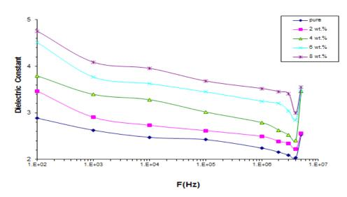
**Fig. 1.** The variation of dielectric constant with the frequency at room temperature. *Egypt.J.Chem.* **62**, Special Issue (Part 2) (2019)
