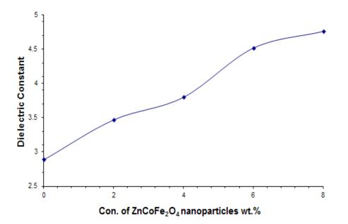
Fig. 3. The variation of dielectric constant for (PS-Cr<sub>2</sub>O<sub>3</sub>) nanocomposites with ZnCoFe<sub>2</sub>O<sub>4</sub> nanoparticles content at 100Hz.
